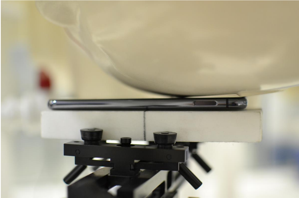
SAR Test Setup Photo 3 – Left Cheek
