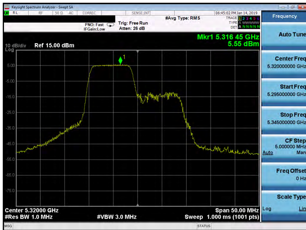
Plot 7-558. Power Spectral Density Plot MIMO ANT2 (20MHz BW 802.11ax – 106 Tones (UNII Band 2A) – Ch. 64)
