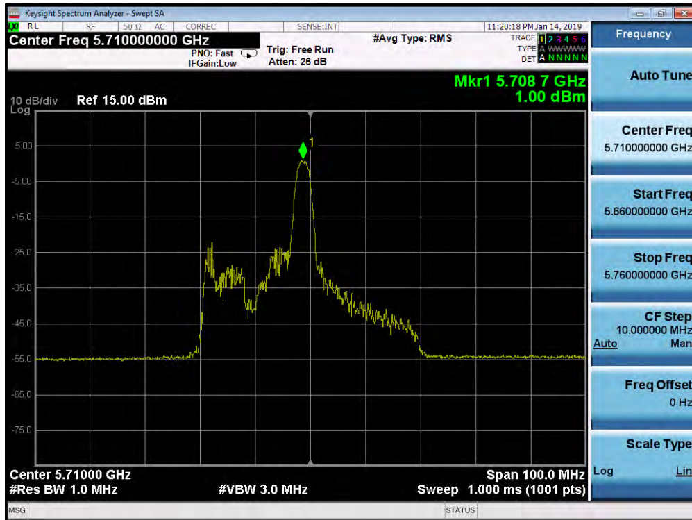
Plot 7-513. Power Spectral Density Plot MIMO ANT2 (40MHz BW 802.11ax – 26 Tones (UNII Band 2C) – Ch. 142)
