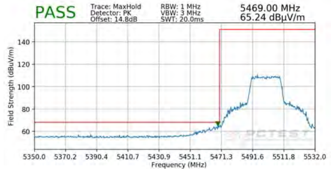
Plot 7-327. Radiated Lower Band Edge Plot SISO ANT2 (Peak – UNII Band 2C)
