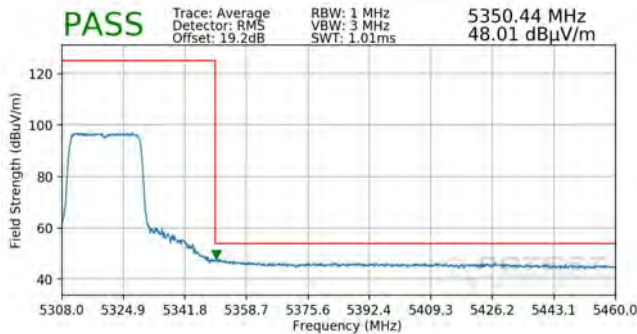
Plot 7-293. Radiated Band Edge Plot SISO ANT1 (Average – WCP)
