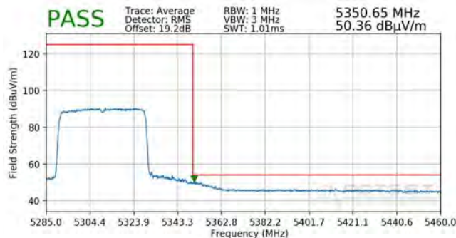
Plot 7-329. Radiated Band Edge Plot SISO ANT2 (Average – WCP)
