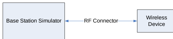
Figure 9-2 Power Measurement Setup
