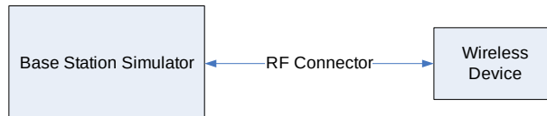
Figure 9-1 Power Measurement Setup
