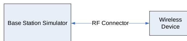
Figure 9-3 Power Measurement Setup
