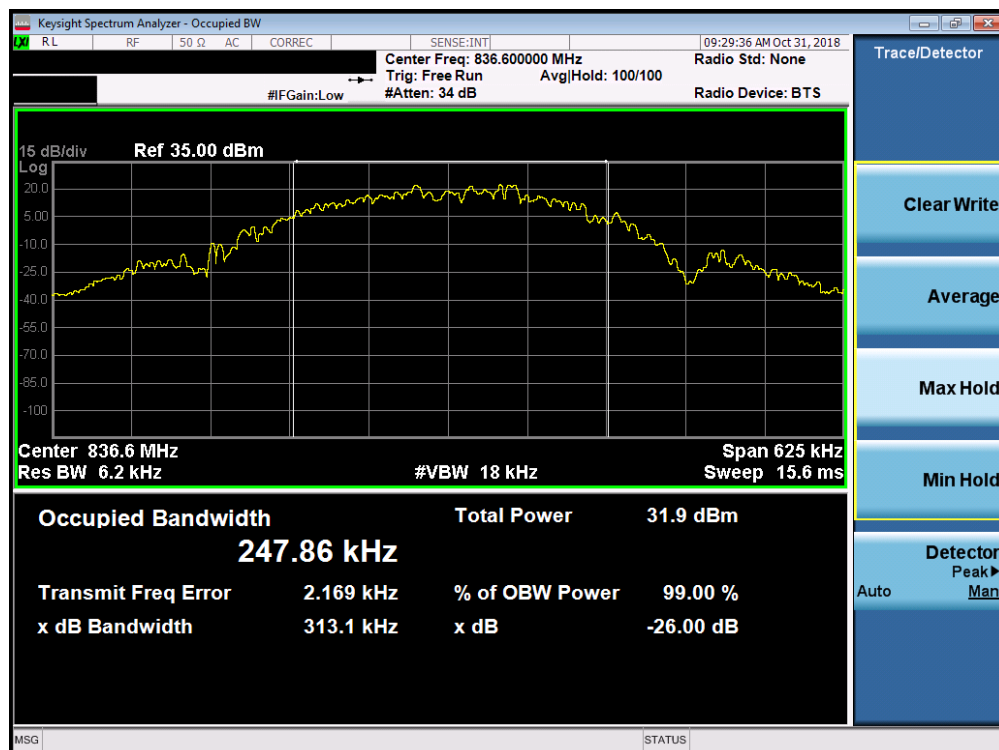
Plot 7-2. Occupied Bandwidth Plot (EDGE850 Mode)
