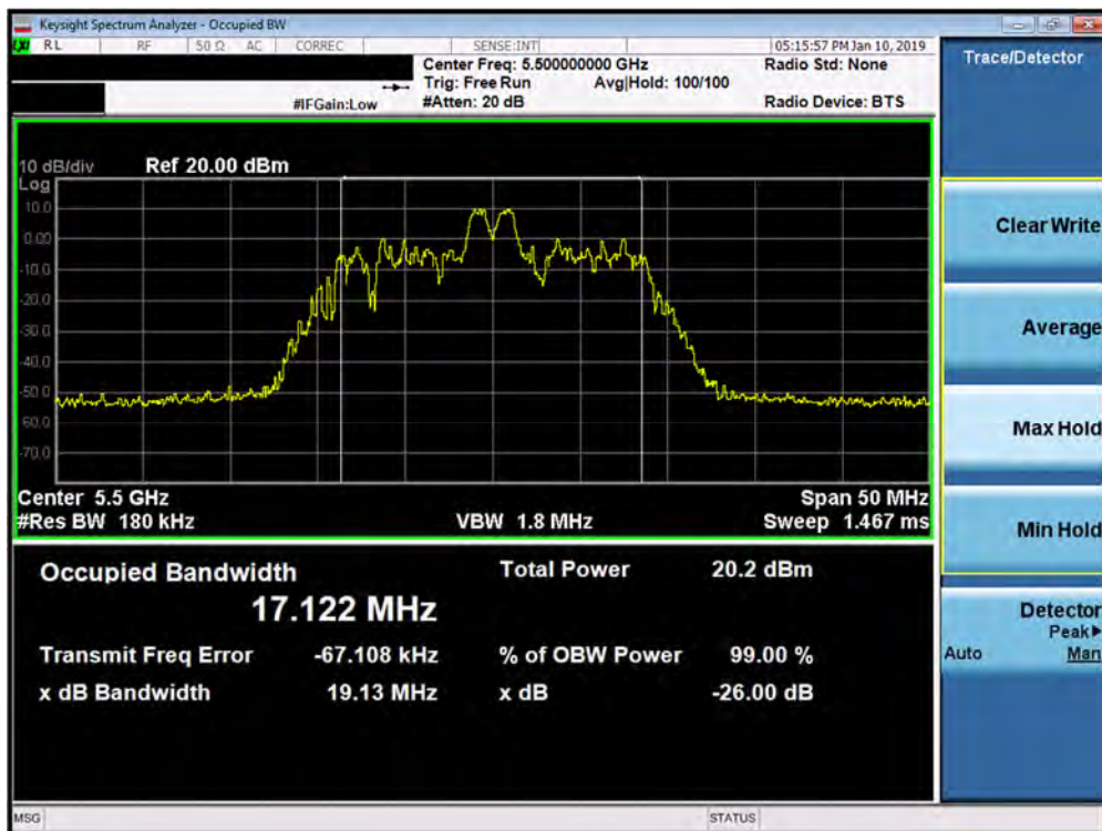
Plot 7-13. 26dB Bandwidth Plot SISO ANT1 (20MHz BW 802.11ax – 26 Tones (UNII Band 2C) – Ch. 100)
