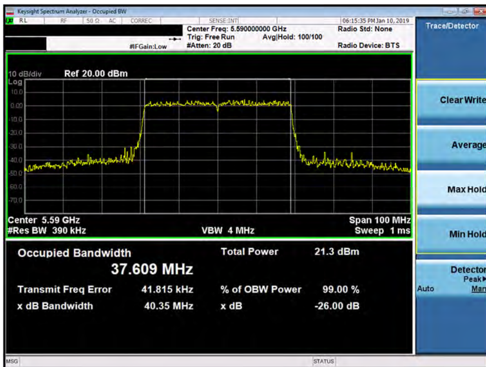
Plot 7-36. 26dB Bandwidth Plot SISO ANT1 (40MHz BW 802.11ax – 484 Tones (UNII Band 2C) – Ch. 118)
