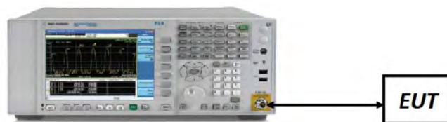
Figure 7-3. Test Instrument & Measurement Setup
