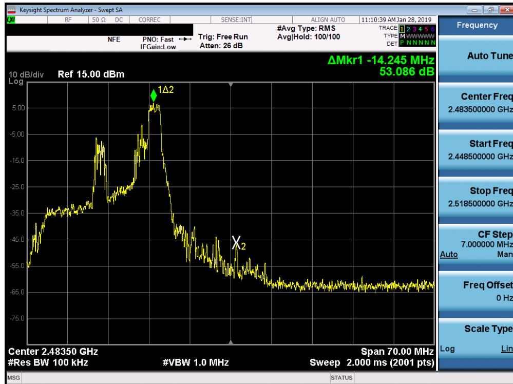
Plot 7-74. Band Edge Plot SISO ANT1 (802.11ax OFDMA – 26 Tones – Ch. 11)
