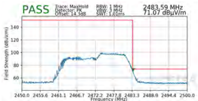
Plot 7-168. Radiated Restricted Upper Band Edge Measurement SISO ANT1 (Peak – 106 Tones)
