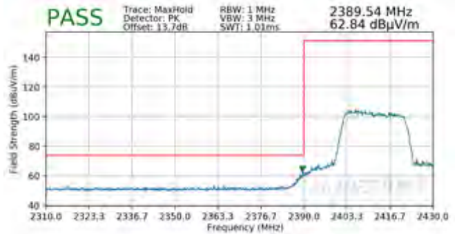
Plot 7-192. Radiated Restricted Lower Band Edge Measurement SISO ANT2 (Peak – 242 Tones)
