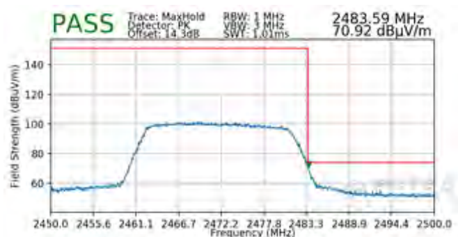
Plot 7-224. Radiated Restricted Upper Band Edge Measurement MIMO (Peak – 242 Tones)
