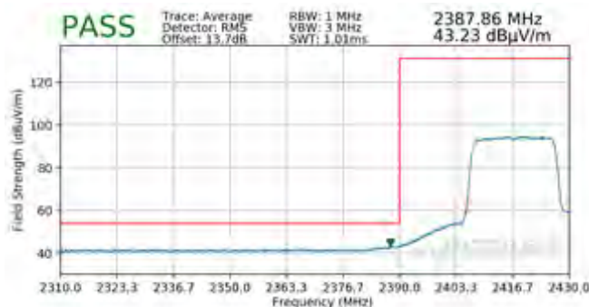
Plot 7-171. Radiated Restricted Lower Band Edge Measurement SISO ANT1 (Average – 242 Tones)
