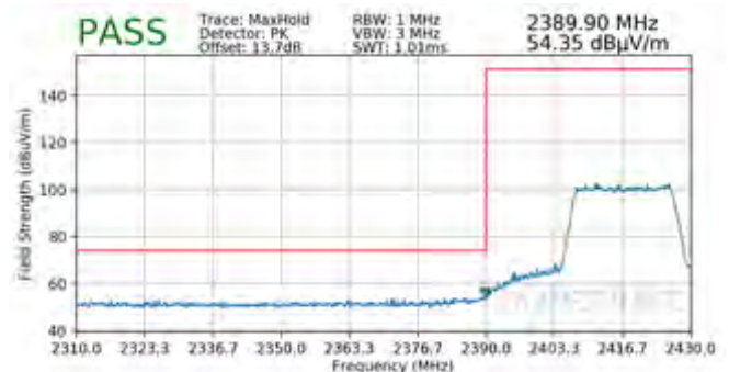
Plot 7-216. Radiated Restricted Lower Band Edge Measurement MIMO (Peak – 242 Tones)
