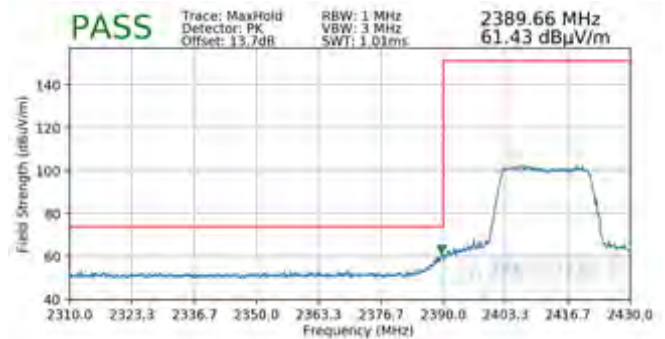
Plot 7-214. Radiated Restricted Lower Band Edge Measurement MIMO (Peak – 242 Tones)
