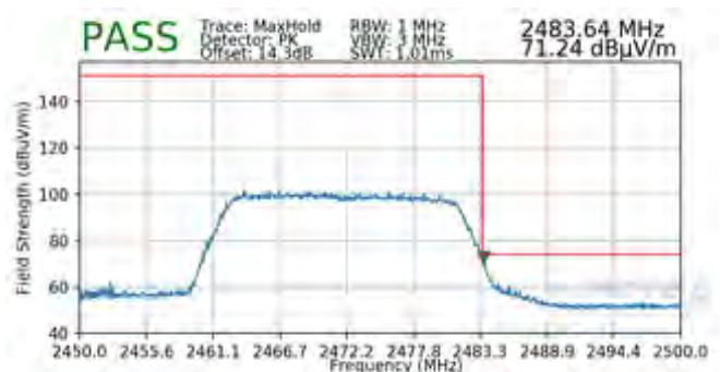
Plot 7-180. Radiated Restricted Upper Band Edge Measurement SISO ANT1 (Peak – 242 Tones)
