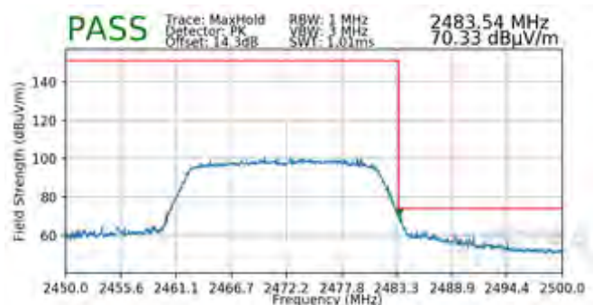
Plot 7-202. Radiated Restricted Upper Band Edge Measurement SISO ANT2 (Peak – 242 Tones)
