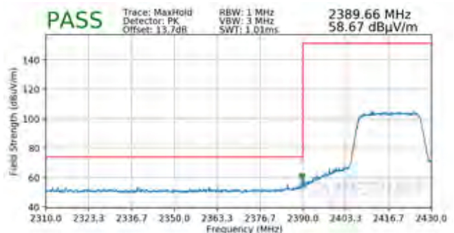
Plot 7-172. Radiated Restricted Lower Band Edge Measurement SISO ANT1 (Peak – 242 Tones)
