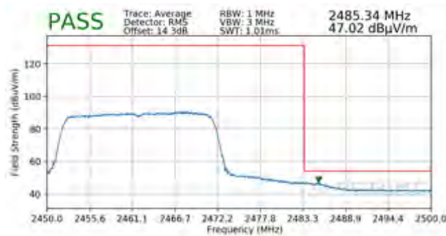
Plot 7-225. Radiated Restricted Band Edge Measurement MIMO with WCP (Average – 242 Tones)
