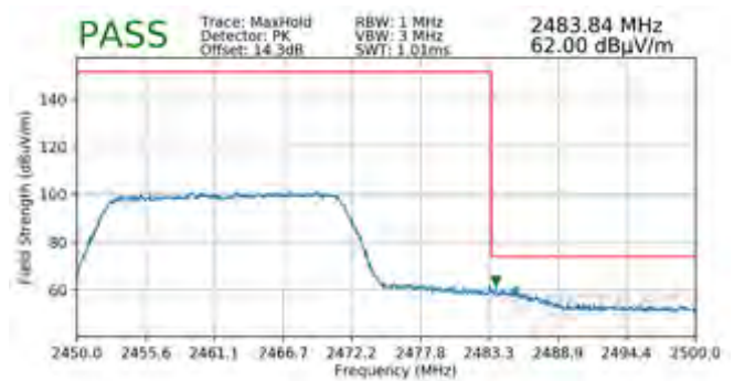
Plot 7-226. Radiated Restricted Band Edge Measurement MIMO with WCP (Peak – 242 Tones)
