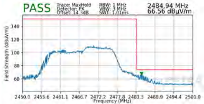
Plot 7-166. Radiated Restricted Upper Band Edge Measurement SISO ANT1 (Peak – 106 Tones)
