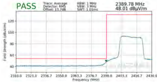
Plot 7-191. Radiated Restricted Lower Band Edge Measurement SISO ANT2 (Average – 242 Tones)
