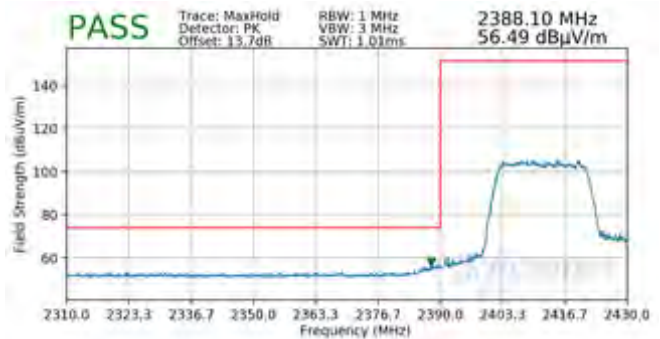
Plot 7-170. Radiated Restricted Lower Band Edge Measurement SISO ANT1 (Peak – 242 Tones)
