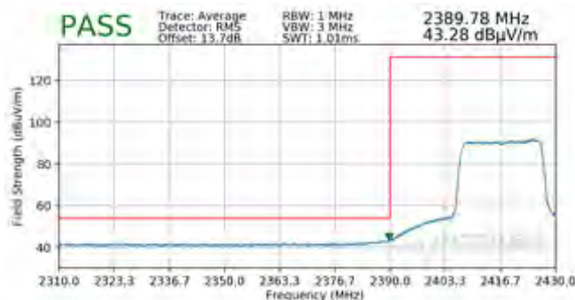
Plot 7-215. Radiated Restricted Lower Band Edge Measurement MIMO (Average – 242 Tones)
