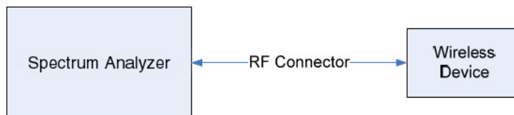
Figure 7-1. Test Instrument & Measurement Setup
