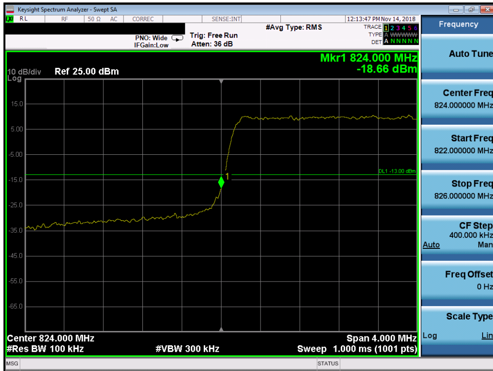
Plot 7-148. Lower Band Edge Plot (Band 26/5 - 3.0MHz QPSK - Full RB Configuration)
