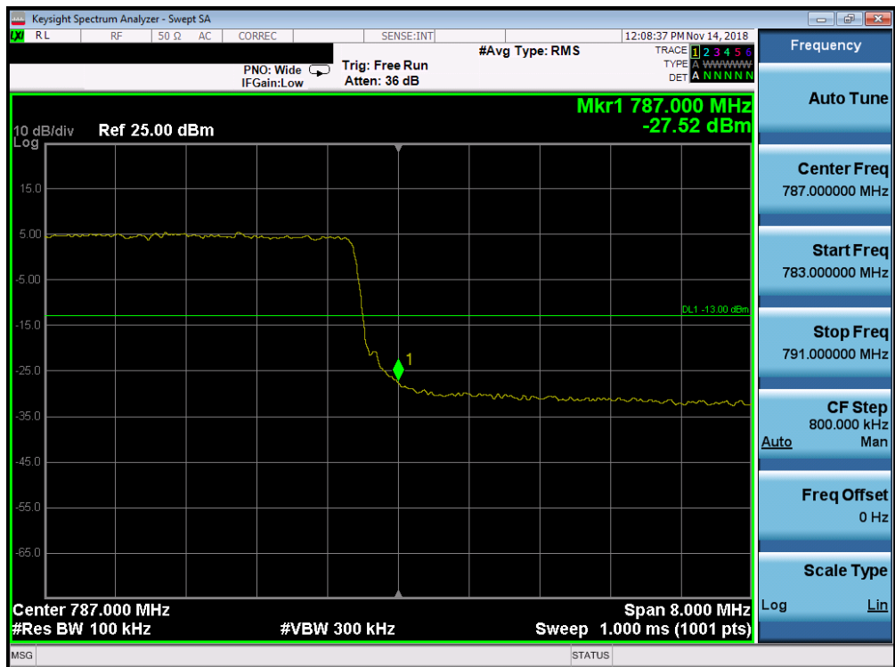
Plot 7-144. Upper Band Edge Plot (Band 13 - 10.0MHz QPSK - Full RB Configuration)
