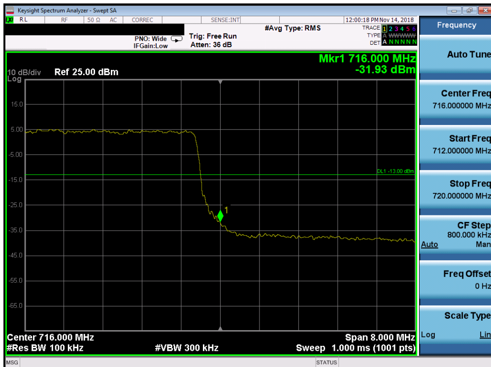
Plot 7-137. Upper Band Edge Plot (Band 12 - 10.0MHz QPSK - Full RB Configuration)
