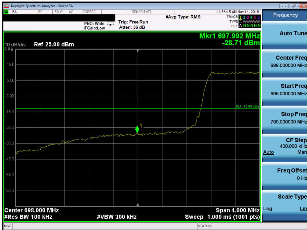
Plot 7-132. Lower Band Edge Plot (Band 12 - 3.0MHz QPSK - Full RB Configuration)
