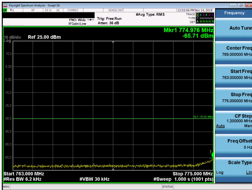
Plot 7-139. Lower Emission Mask Plot (Band 13 - 5.0MHz QPSK - Full RB Configuration)
