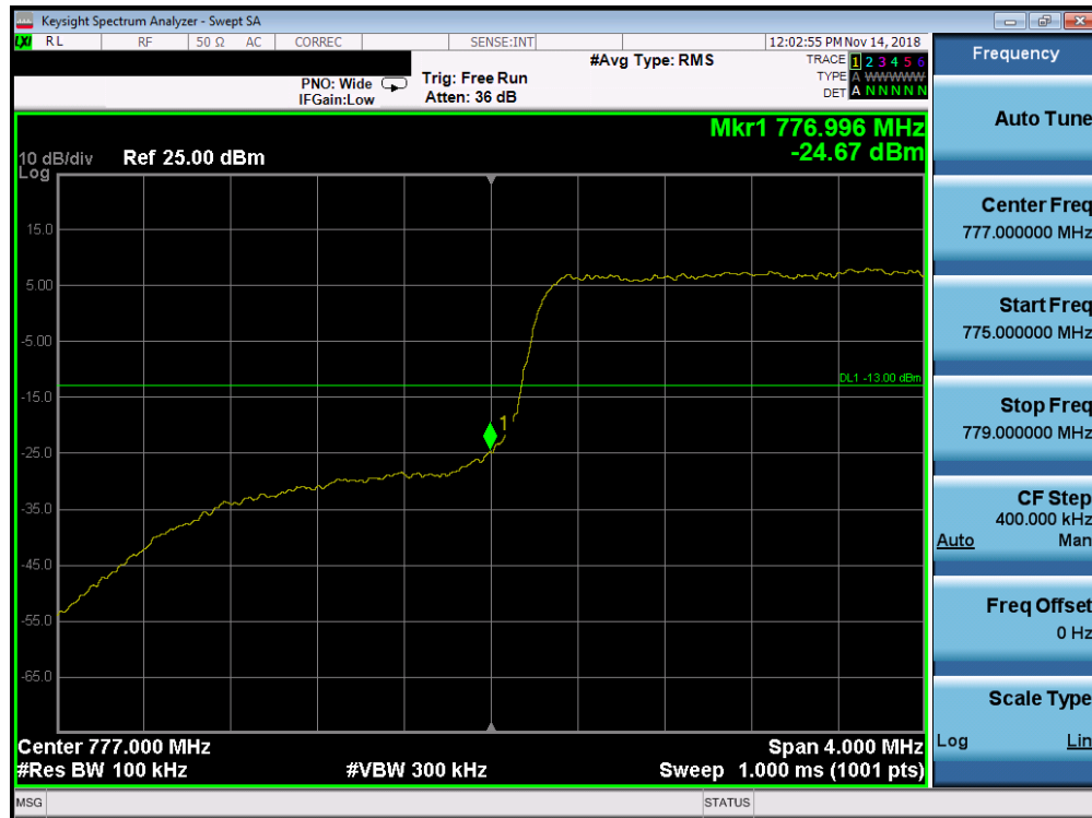
Plot 7-138. Lower Band Edge Plot (Band 13 - 5.0MHz QPSK - Full RB Configuration)
