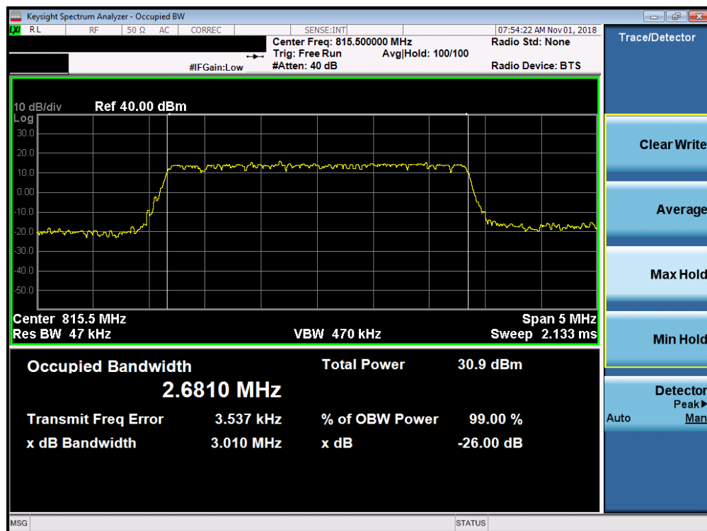
Plot 7-5. Occupied Bandwidth Plot (LTE Band 26, 3MHz 16-QAM – RB Size 15– Low Channel)
