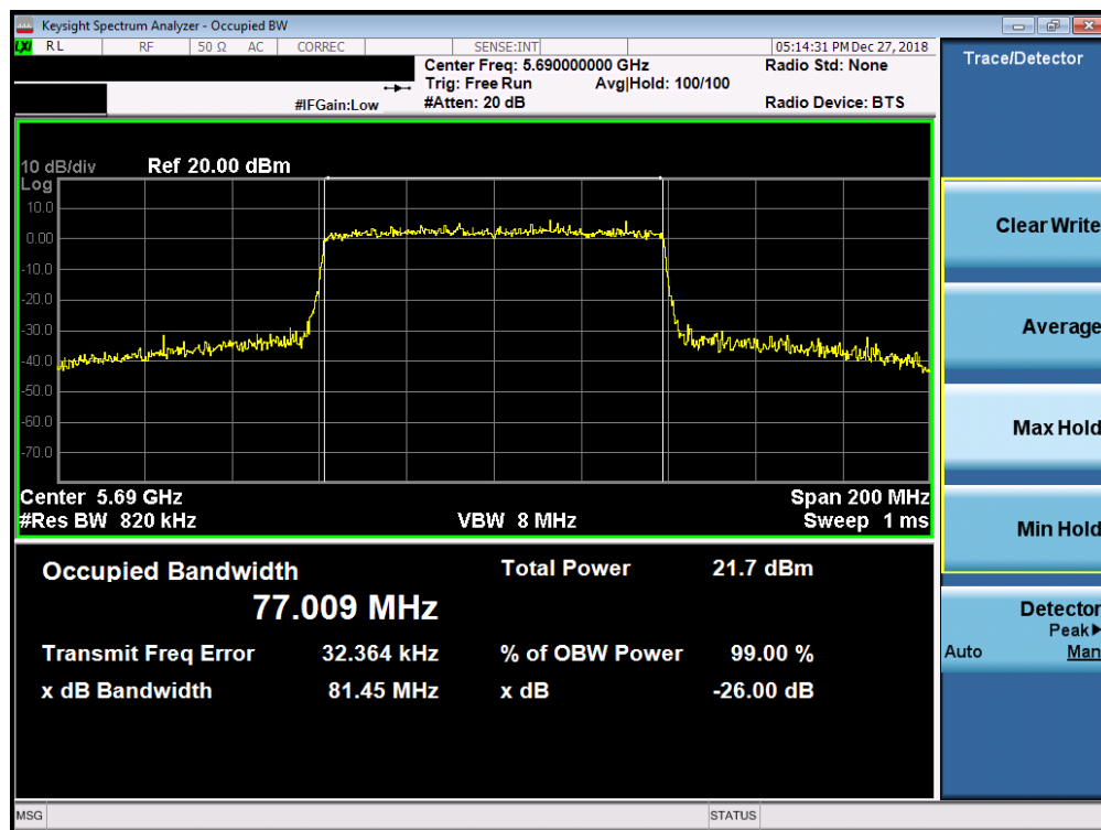
Plot 7-51. 26dB Bandwidth Plot SISO ANT1 (80MHz BW 802.11ac (UNII Band 2C) – Ch. 138)
