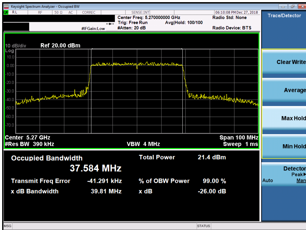
Plot 7-78. 26dB Bandwidth Plot SISO ANT2 (40MHz BW 802.11ax (UNII Band 2A) – Ch. 54)
