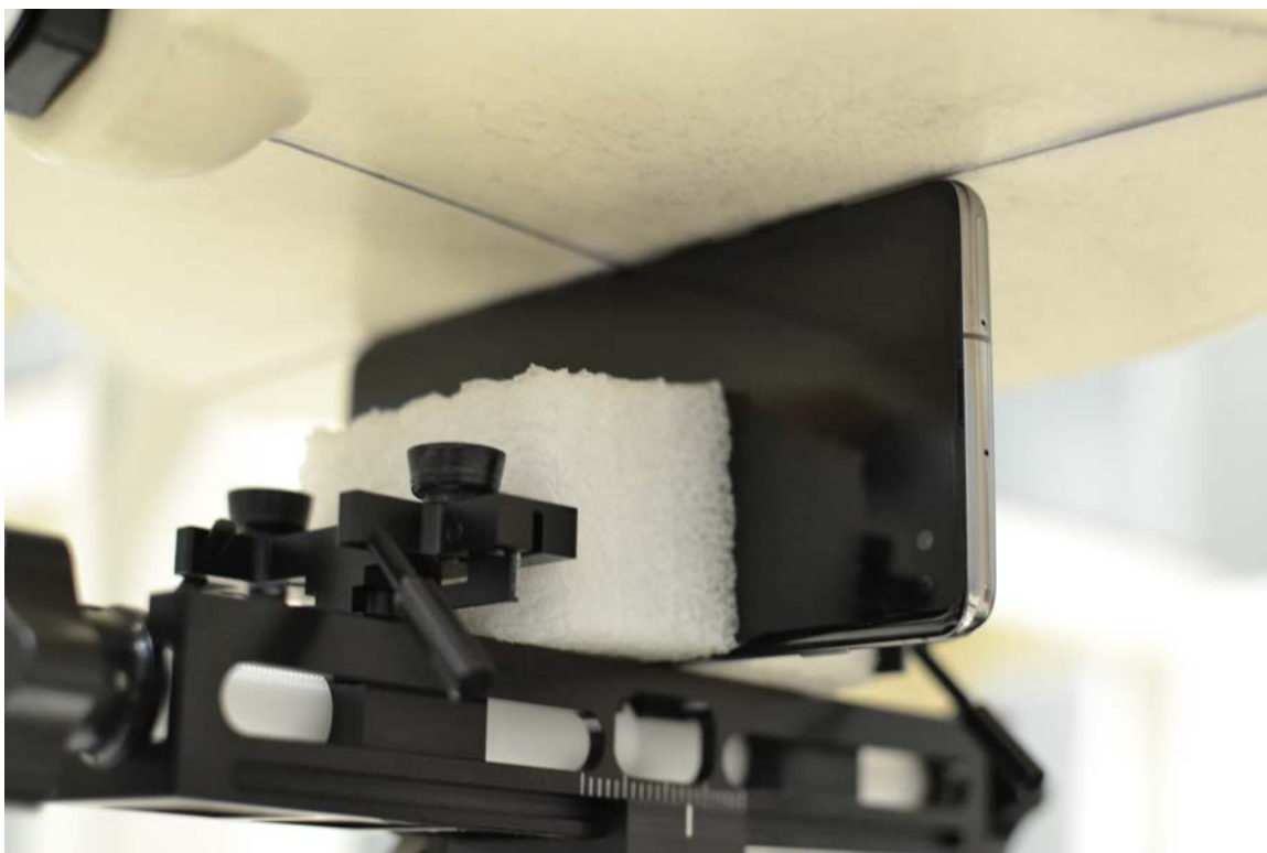
SAR Test Setup Photo 21 – Left Side at 0 mm
