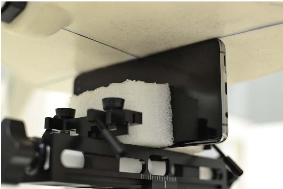
SAR Test Setup Photo 19 – Right Side at 0 mm
