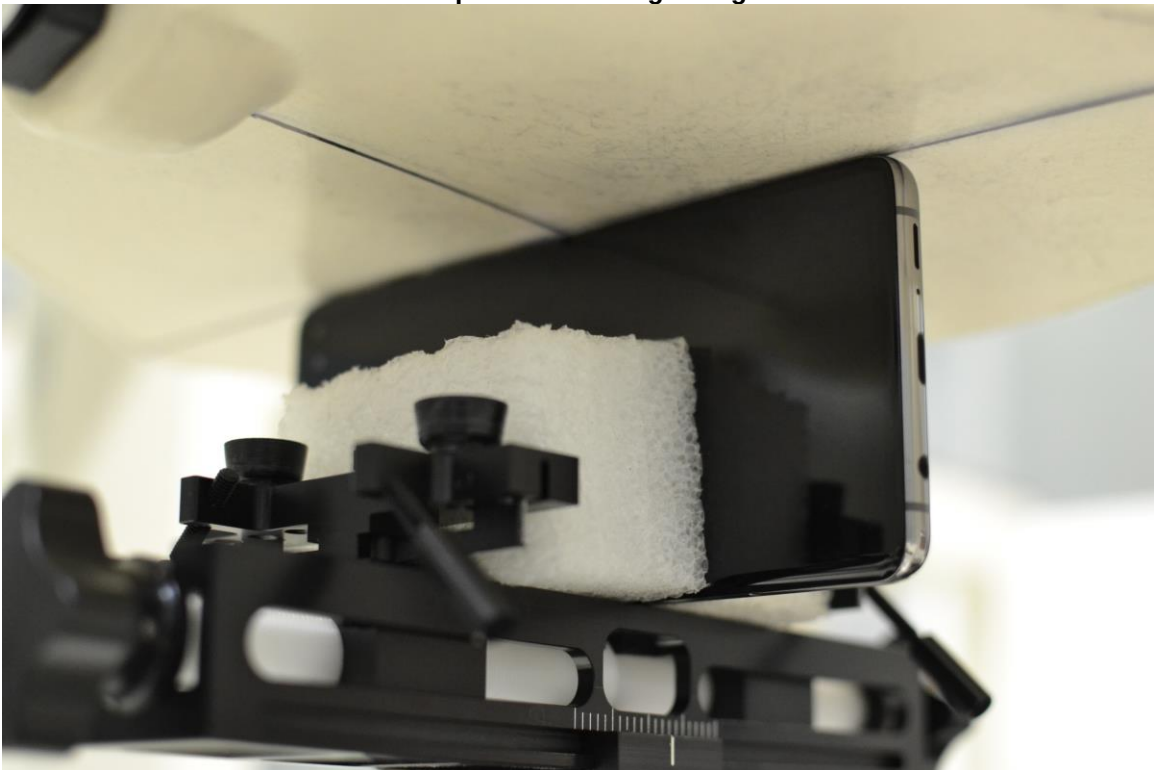
SAR Test Setup Photo 18 – Right Edge at 0 mm
