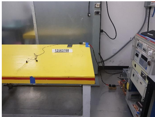
AC LINE CONDUCTED (FRONT)
