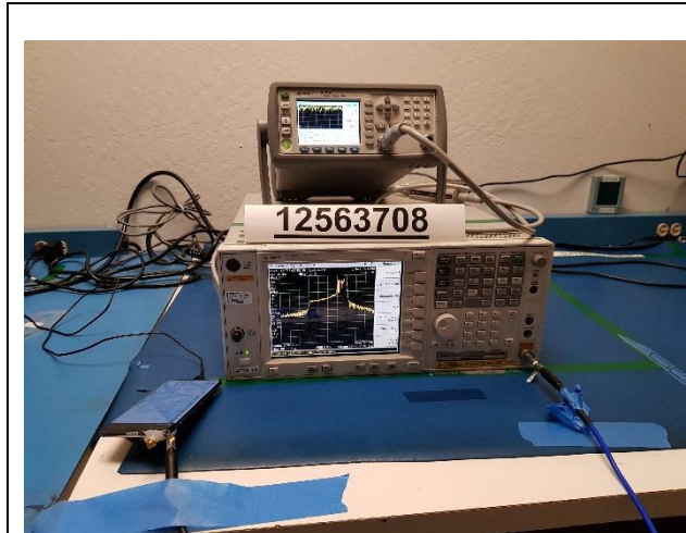
RF ANTENNA PORT CONDUCTED
