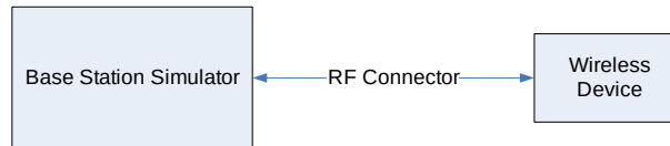
Figure 9-4 Power Measurement Setup
