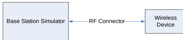
Figure 9-1 Power Measurement Setup
