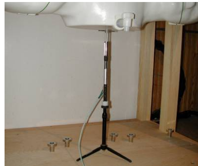
Figure 10-2 System Verification Setup Photo
