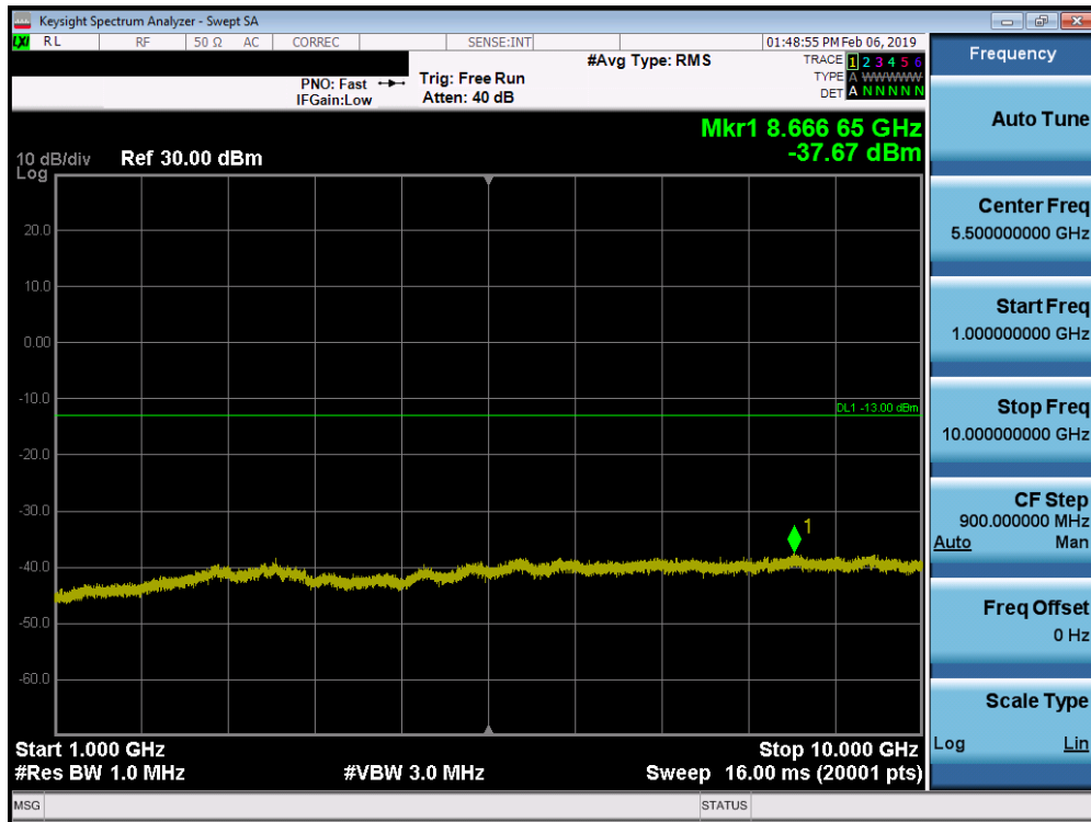
Plot 7-18. Conducted Spurious Plot (LTE Band 26, 10.0MHz QPSK – RB Size 1, RB Offset 0)
