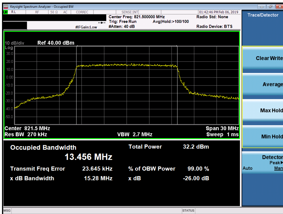
Plot 7-13. Occupied Bandwidth Plot (LTE Band 26, 15MHz QPSK – RB Size 75)
