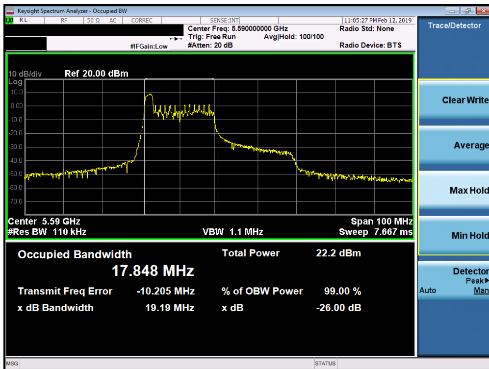
Plot 7-38. 26dB Bandwidth Plot SISO ANT2 (40MHz BW 802.11ax – 26 Tones (UNII Band 2C) – Ch. 118)
