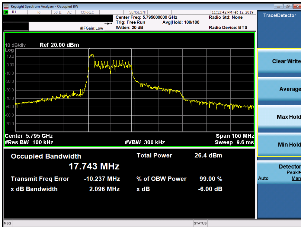
Plot 7-53. 6dB Bandwidth Plot SISO ANT2 (40MHz BW 802.11ax – 26 Tones (UNII Band 3) – Ch. 159)
