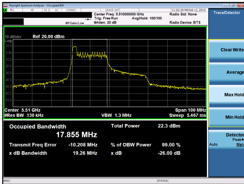
Plot 7-37. 26dB Bandwidth Plot SISO ANT2 (40MHz BW 802.11ax – 26 Tones (UNII Band 2C) – Ch. 102)
