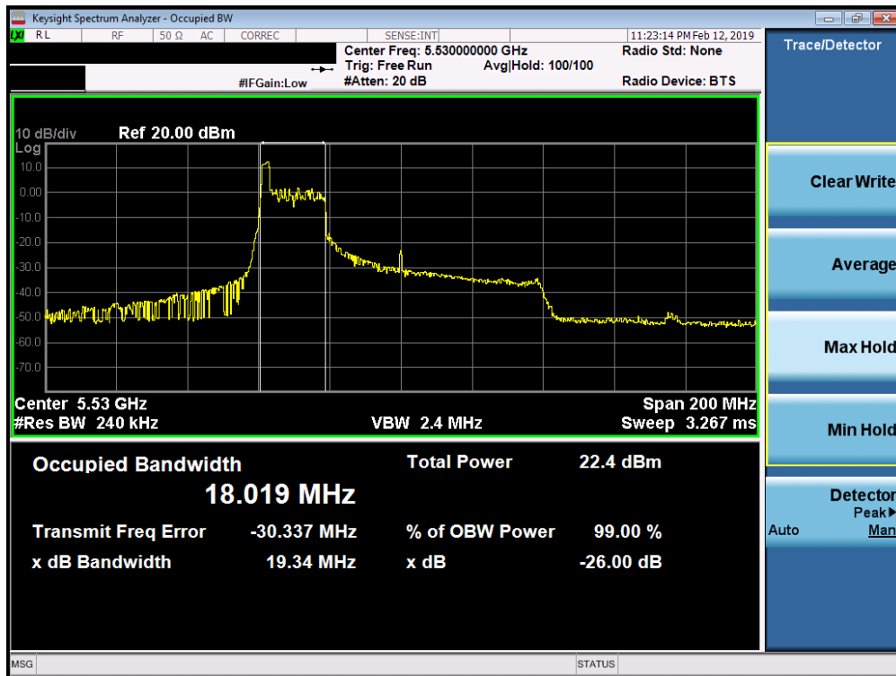
Plot 7-40. 26dB Bandwidth Plot SISO ANT2 (80MHz BW 802.11ax – 26 Tones (UNII Band 2C) – Ch. 106)
