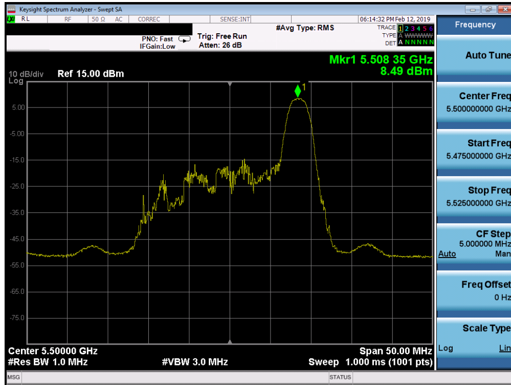
Plot 7-67. Power Spectral Density Plot SISO ANT1 (20MHz BW 802.11ax – 26 Tones (UNII Band 2C) – Ch. 100)
