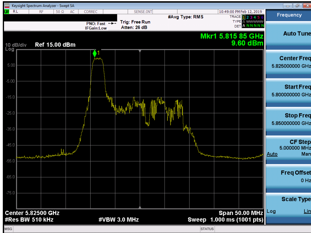
Plot 7-105. Power Spectral Density Plot SISO ANT2 (20MHz BW 802.11ax – 26 Tones (UNII Band 3) – Ch. 165)
