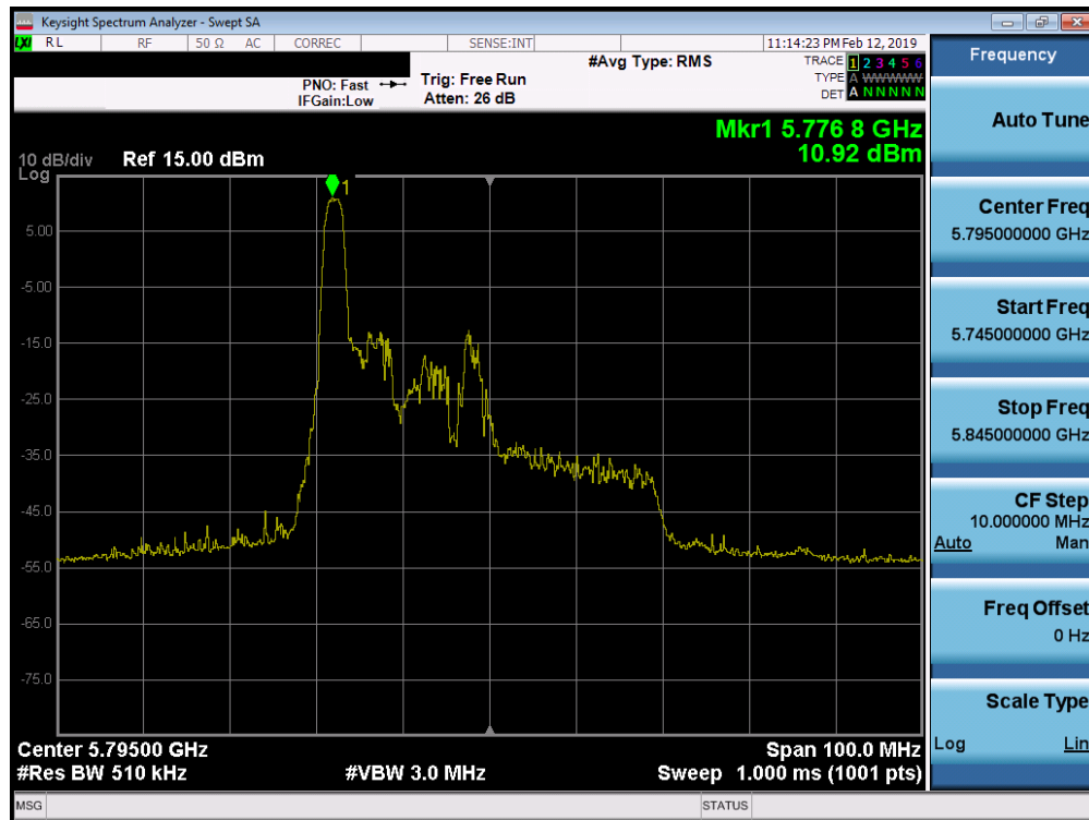
Plot 7-107. Power Spectral Density Plot SISO ANT2 (40MHz BW 802.11ax – 26 Tones (UNII Band 3) – Ch. 159)
