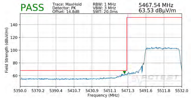
Plot 7-241. Radiated Lower Band Edge Plot MIMO (Peak – UNII Band 2C – 484 Tones)
