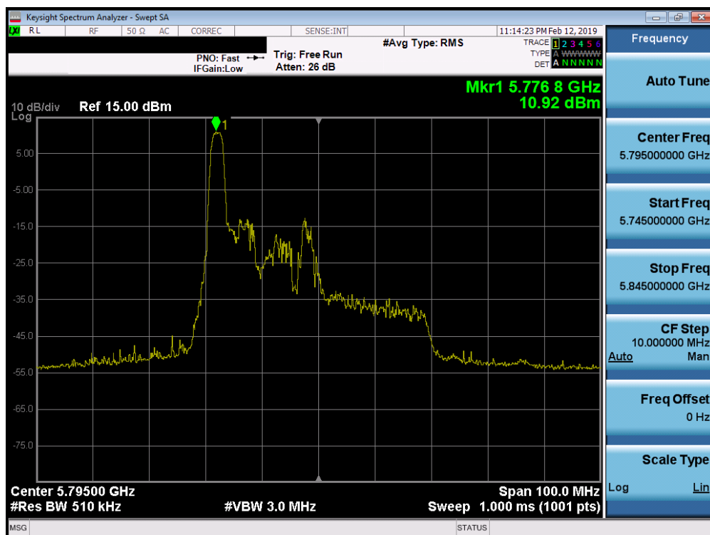
Plot 7-161. Power Spectral Density Plot MIMO ANT2 (40MHz BW 802.11ax – 26 Tones (UNII Band 3) – Ch. 159)
