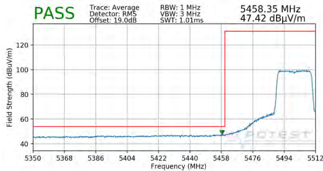
Plot 7-212. Radiated Lower Band Edge Plot SISO ANT2 (Average – UNII Band 2C – 242 Tones)
