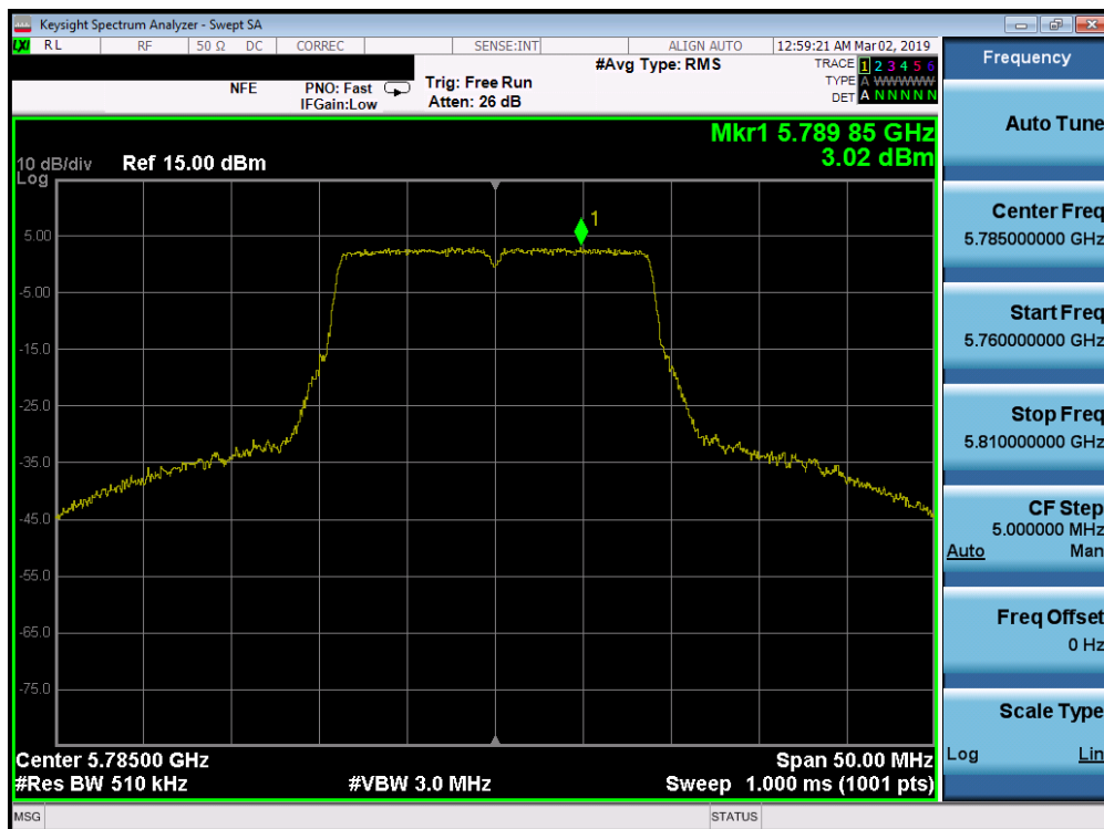
Plot 7-227. Power Spectral Density Plot SISO ANT2 (20MHz BW 802.11n (UNII Band 3) – Ch. 157)
