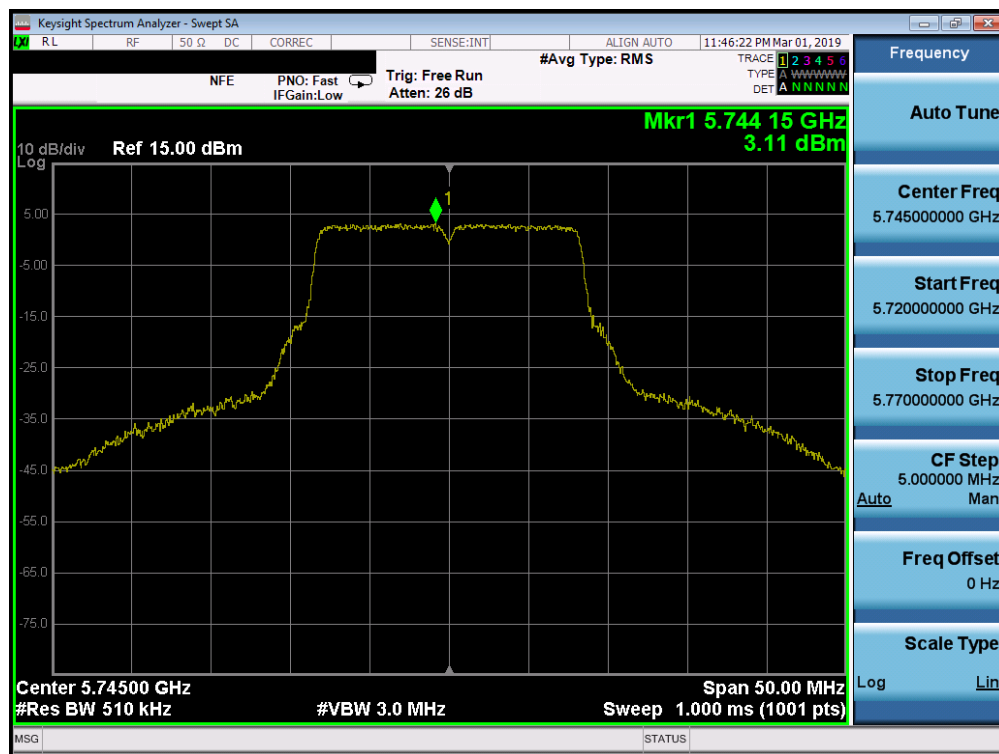
Plot 7-172. Power Spectral Density Plot SISO ANT1 (802.11a (UNII Band 3) – Ch. 149)
