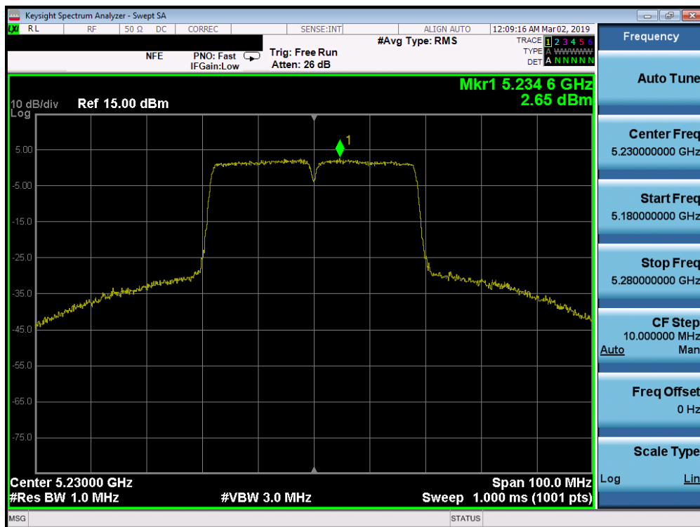
Plot 7-143. Power Spectral Density Plot SISO ANT1 (40MHz BW 802.11n (UNII Band 1) – Ch. 46)
