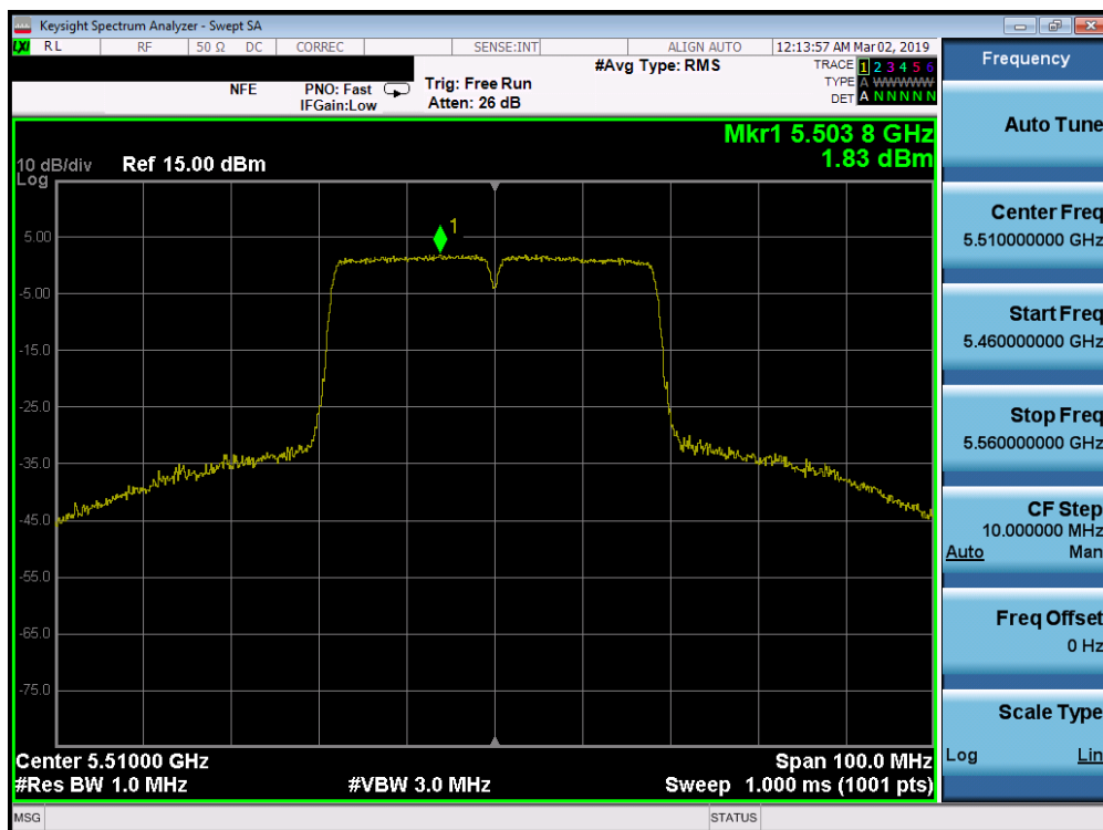
Plot 7-166. Power Spectral Density Plot SISO ANT1 (40MHz BW 802.11n (UNII Band 2C) – Ch. 102)
