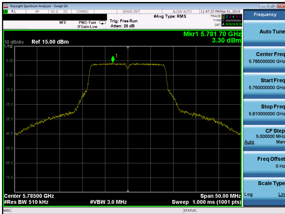
Plot 7-173. Power Spectral Density Plot SISO ANT1 (802.11a (UNII Band 3) – Ch. 157)
