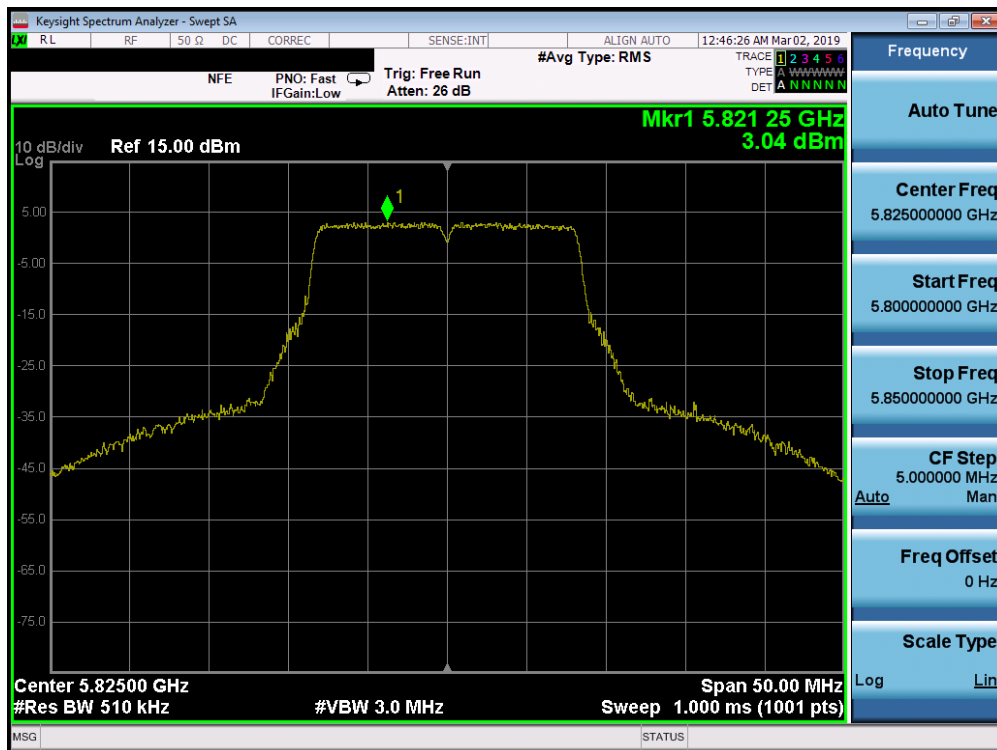
Plot 7-225. Power Spectral Density Plot SISO ANT2 (802.11a (UNII Band 3) – Ch. 165)
