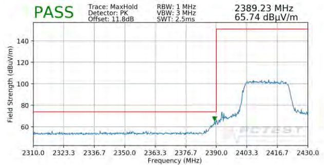
Plot 7-100. Radiated Restricted Lower Band Edge Measurement SISO ANT2 (Peak – 242 Tones)
