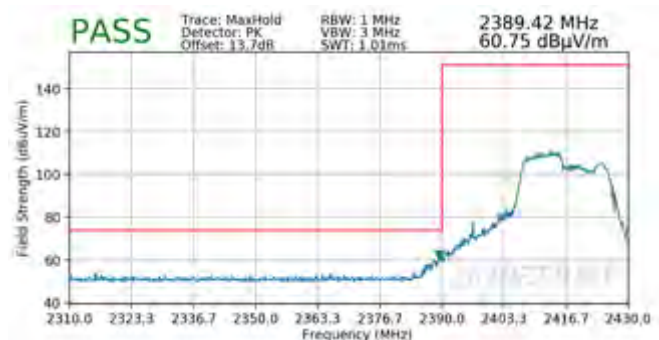
Plot 7-66. Radiated Restricted Lower Band Edge Measurement SISO ANT1 (Peak – 106 Tones)
