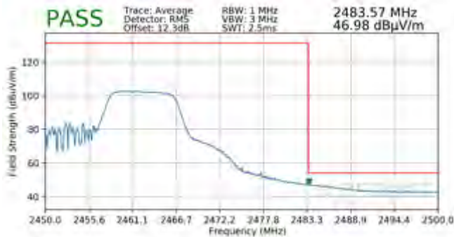
Plot 7-67. Radiated Restricted Upper Band Edge Measurement SISO ANT1 (Average – 106 Tones)
