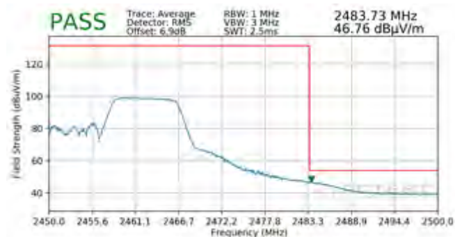
Plot 7-115. Radiated Restricted Upper Band Edge Measurement MIMO (Average – 106 Tones)
