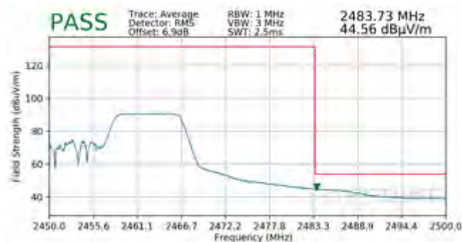
Plot 7-91. Radiated Restricted Lower Band Edge Measurement SISO ANT2 (Average – 106 Tones)
