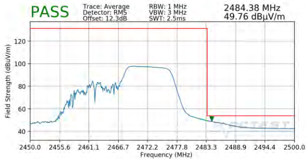
Plot 7-119. Radiated Restricted Upper Band Edge Measurement MIMO (Average – 106 Tones)
