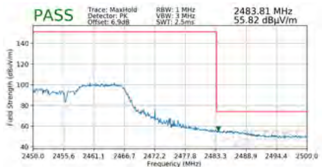
Plot 7-92. Radiated Restricted Lower Band Edge Measurement SISO ANT2 (Peak – 106 Tones)
