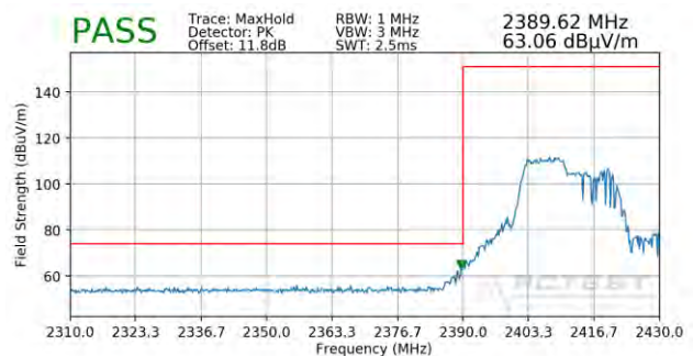
Plot 7-64. Radiated Restricted Lower Band Edge Measurement SISO ANT1 (Peak – 106 Tones)
