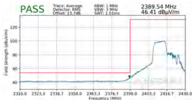
Plot 7-65. Radiated Restricted Lower Band Edge Measurement SISO ANT1 (Average – 106 Tones)
