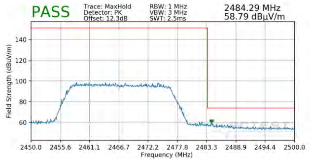
Plot 7-108. Radiated Restricted Band Edge Measurement SISO ANT2 with WCP (Peak – 242 Tones)
