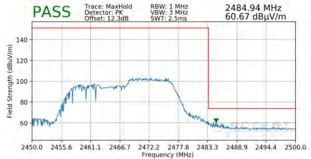
Plot 7-96. Radiated Restricted Upper Band Edge Measurement SISO ANT2 (Peak – 106 Tones)
