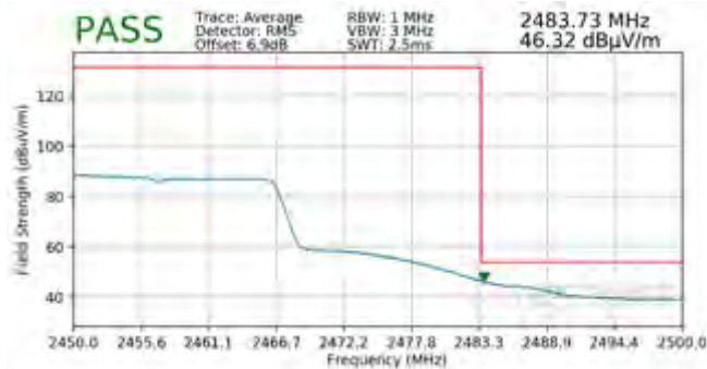
Plot 7-103. Radiated Restricted Upper Band Edge Measurement SISO ANT2 (Average – 242 Tones)
