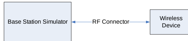
Figure 9-4 Power Measurement Setup
