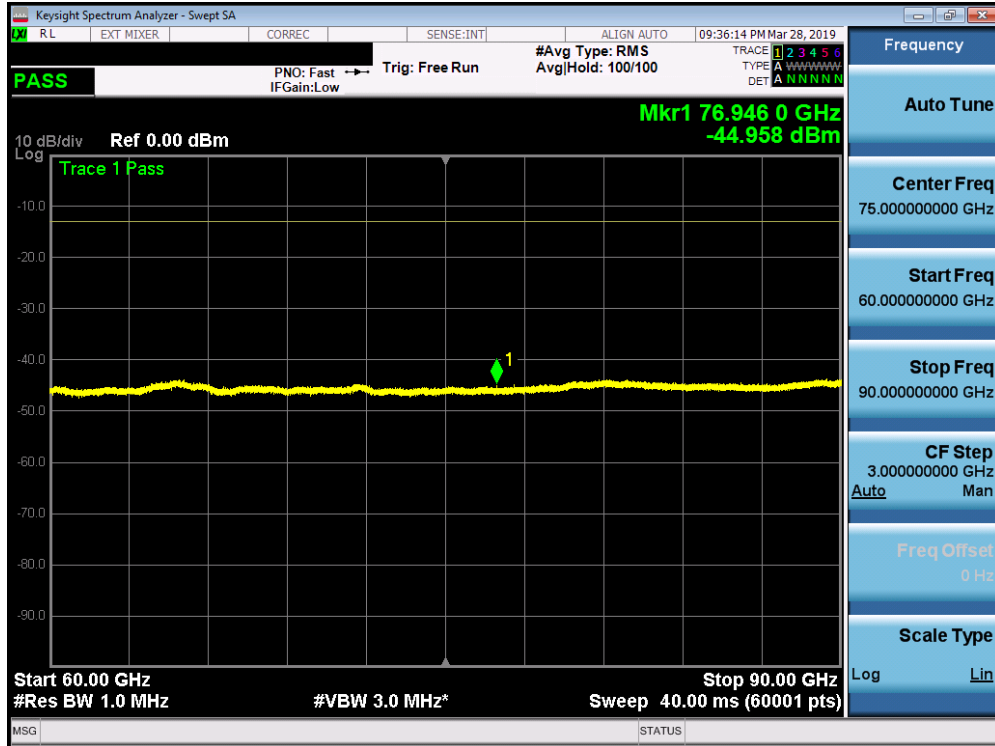
Plot 7-109. J Patch Radiated Spurious Plot 60-90 GHz (1CC QPSK Mid Channel V Beam)
