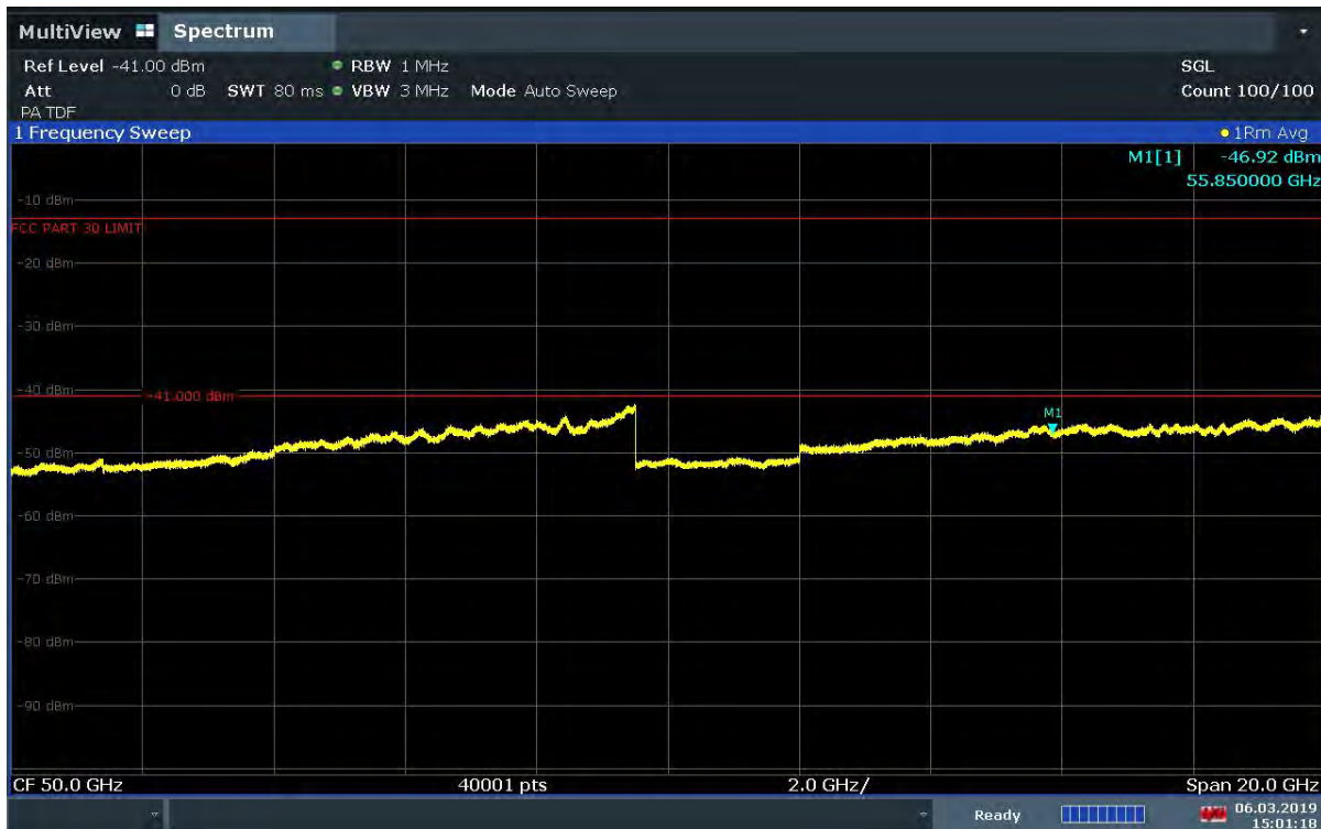
Plot 7-103. J Patch Radiated Spurious Plot 40-60 GHz (1CC 16QAM Mid Channel V Beam)
