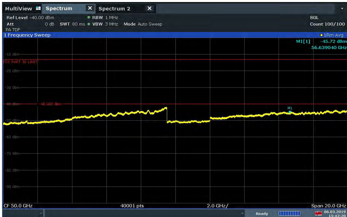
Plot 7-104. J Patch Radiated Spurious Plot 40-60 GHz (1CC 16QAM High Channel V Beam)
