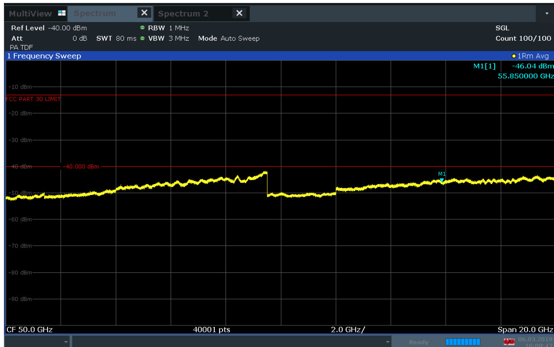
Plot 7-69. J Dipole Radiated Spurious Plot 40-60 GHz (1CC 16QAM Mid Channel V Beam)
