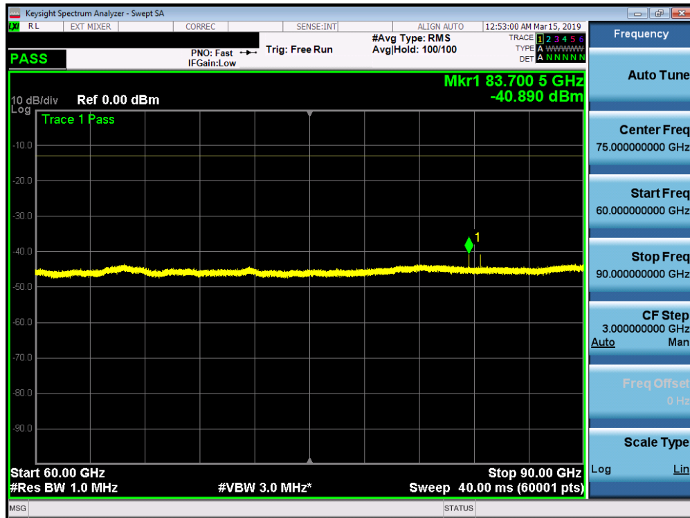
Plot 7-143. K Patch Radiated Spurious Plot 60-90 GHz (1CC QPSK Mid Channel V Beam)
