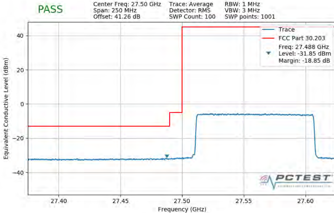
Plot 7-349. Lower Band Edge Plot (1CC 100MHz QPSK Full RB)
