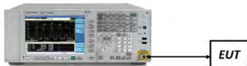
Figure 7-4. Test Instrument & Measurement Setup
