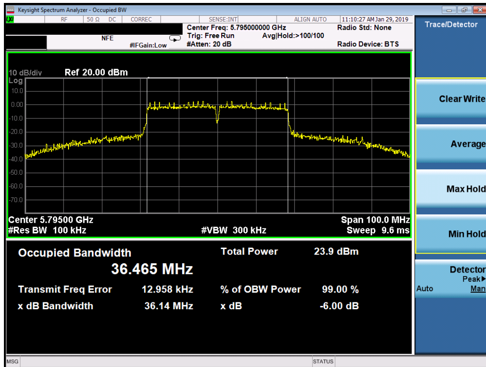
Plot 7-128. 6dB Bandwidth Plot SISO ANT2 (40MHz BW 802.11n (UNII Band 3) – Ch. 159)
