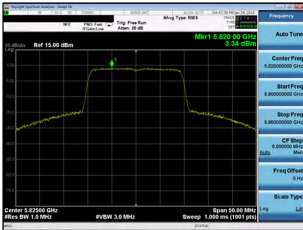
Plot 7-192. Power Spectral Density Plot SISO ANT1 (20MHz BW 802.11ax (UNII Band 3) – Ch. 165)
