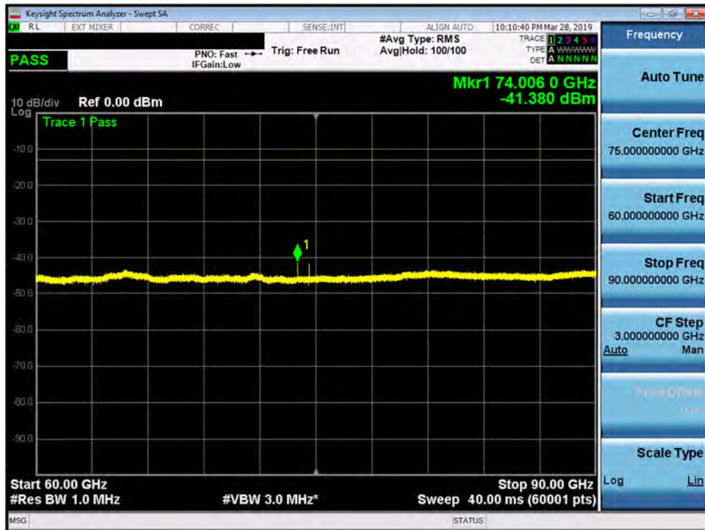
Plot 7-185. L Patch Radiated Spurious Plot 60-90 GHz (1CC QPSK Low Channel H Beam)
