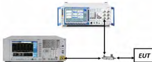
Figure 7-2. Test Instrument & Measurement Setup
