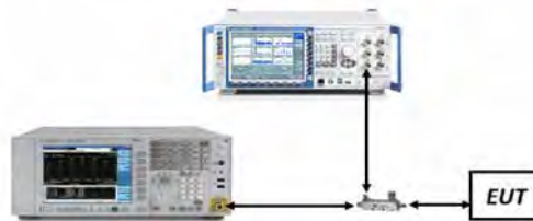
Figure 7-4. Test Instrument & Measurement Setup
