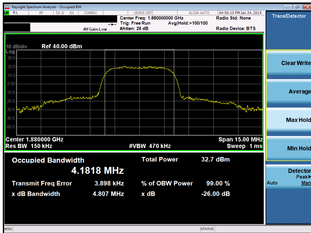
Plot 7-9. Occupied Bandwidth Plot (PCS WCDMA Mode)
