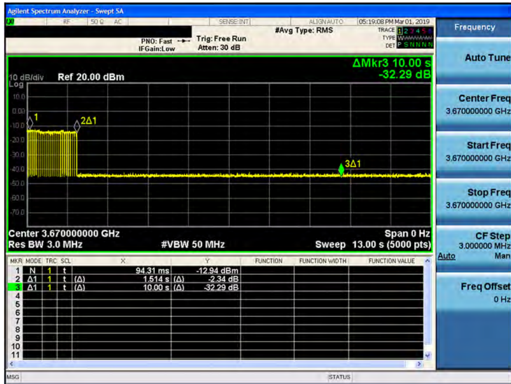
Plot 7-46. Run#2 End User Device Discontinues Operations within 10s
