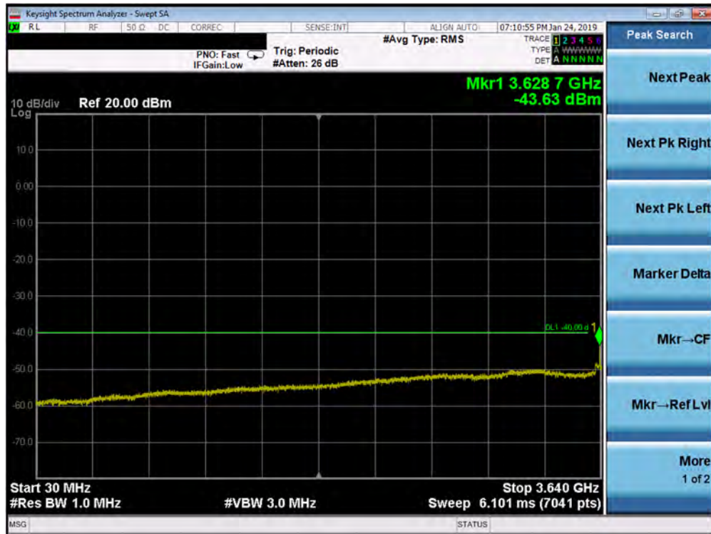
Plot 7-23. Conducted Spurious Plot (Band 48 - 20.0MHz QPSK - RB Size 1, RB Offset 0 - High Channel)
