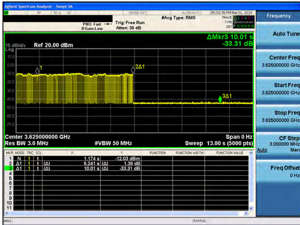
Plot 7-44. Run#1 End User Device Discontinues Operations within 10s
