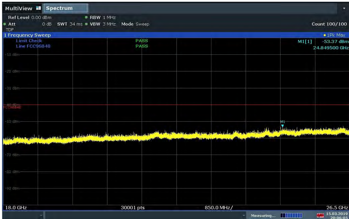
Plot 7-39. Radiated Spurious Plot 18 - 26.5GHz (Band 48 Ant Pol H)
