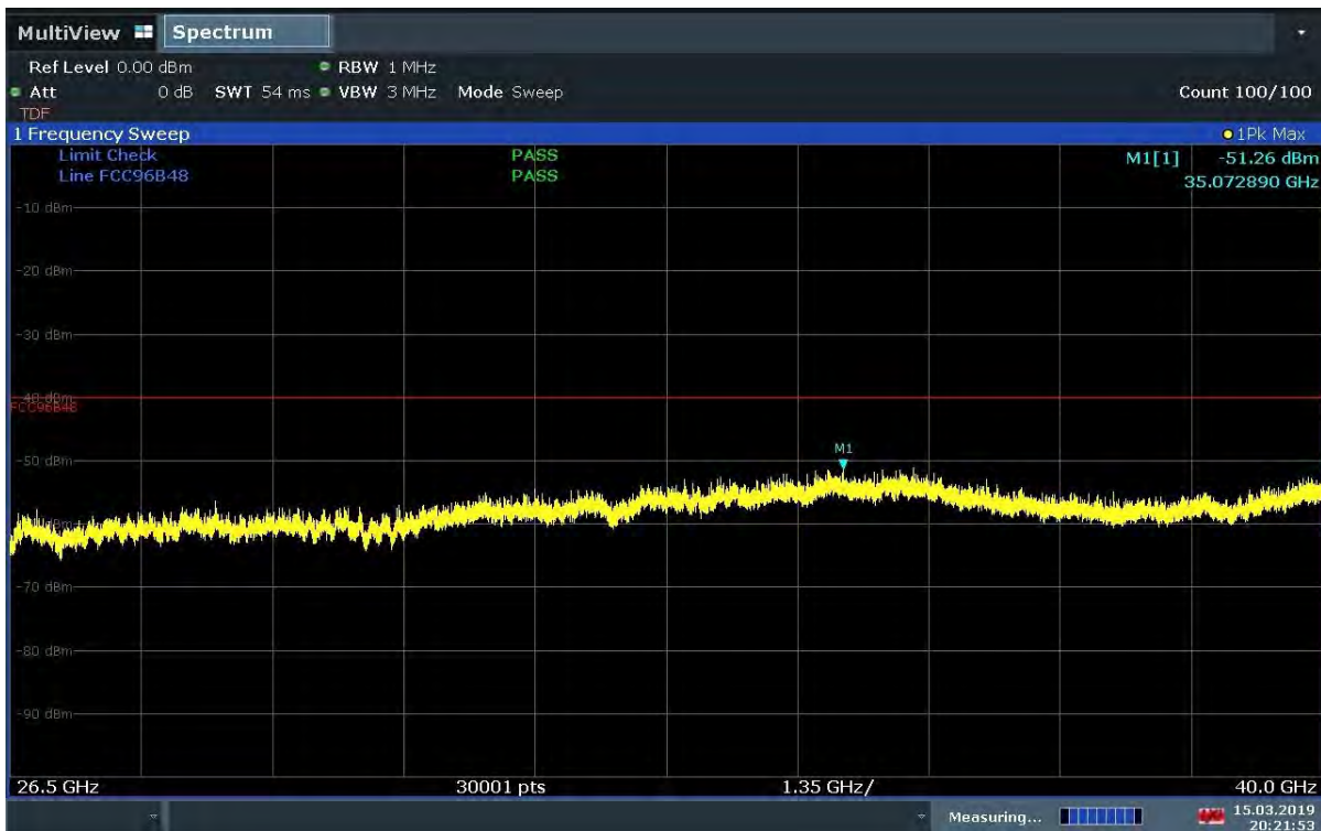
Plot 7-41. Radiated Spurious Plot 26.5 - 40GHz (Band 48 Ant Pol H)
