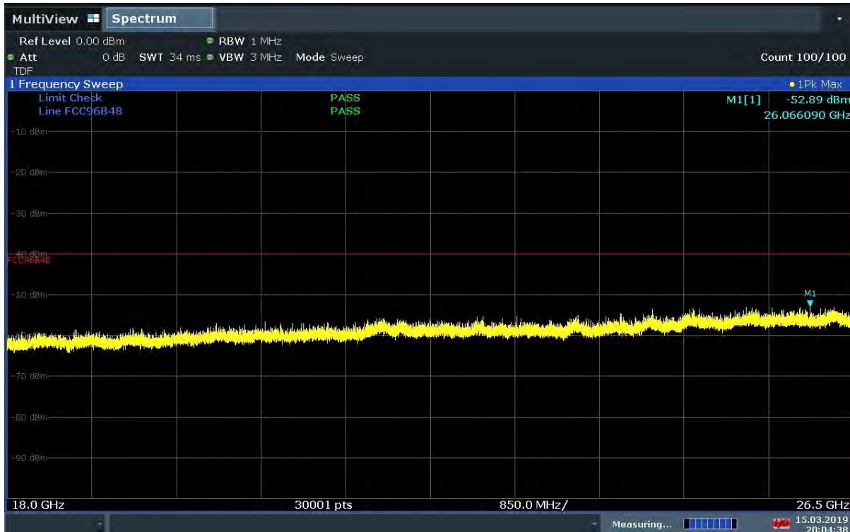
Plot 7-40. Radiated Spurious Plot 18 - 26.5GHz (Band 48 Ant Pol V)
