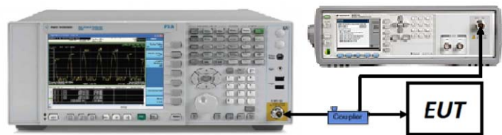
Figure 7-6. Test Instrument & Measurement Setup
