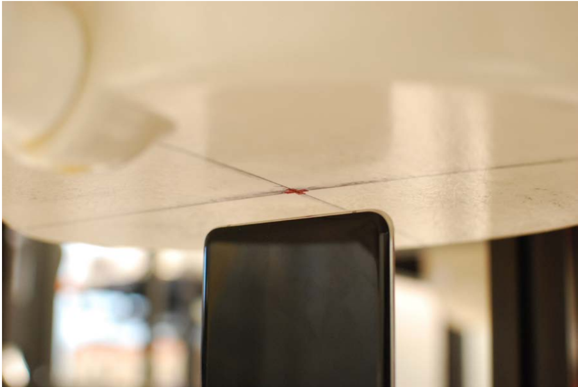
SAR Test Setup Photo 15 – Bottom Side at 9 mm
