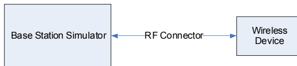
Figure 9-1 Power Measurement Setup
