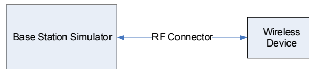
Figure 9-3 Power Measurement Setup
