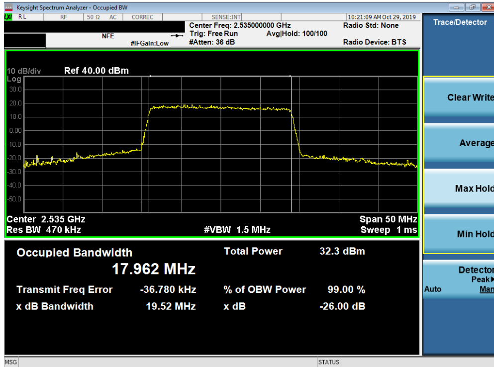
Plot 7-129. Occupied Bandwidth Plot (Band 7 - 20.0MHz QPSK - Full RB Configuration)
