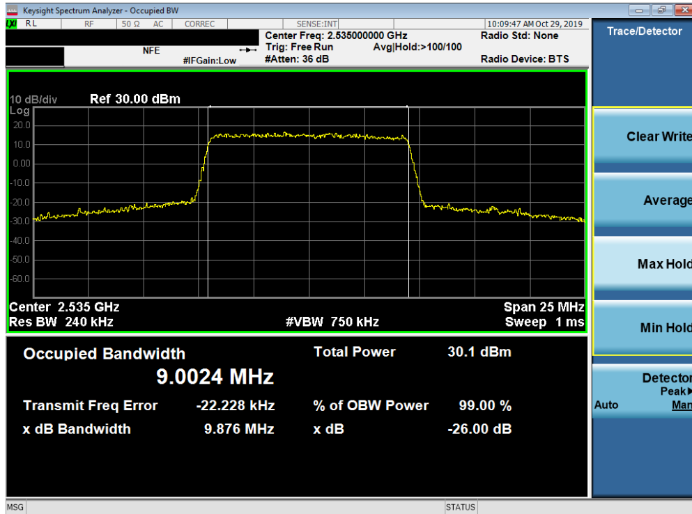
Plot 7-123. Occupied Bandwidth Plot (Band 7 - 10.0MHz 64-QAM - Full RB Configuration)
