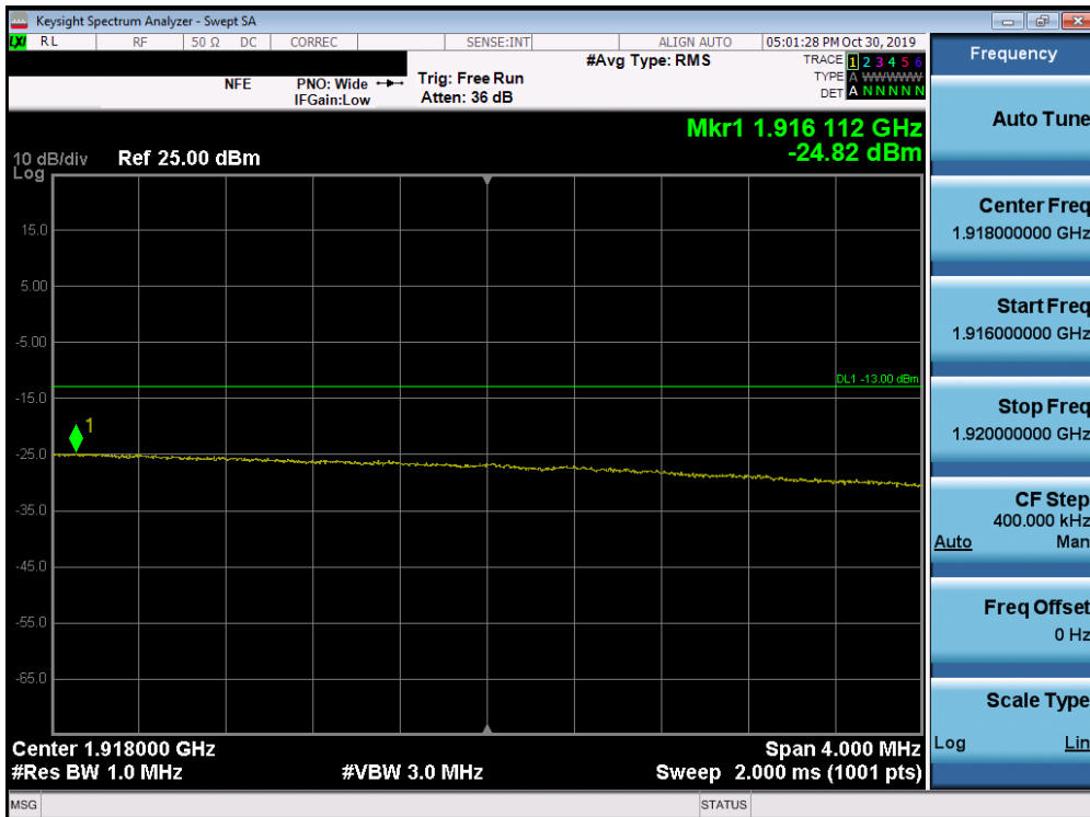
Plot 7-348. Upper Extended Band Edge Plot (Band 25 - 20.0MHz QPSK - Full RB Configuration)
