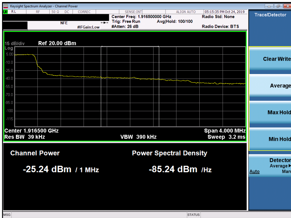
Plot 7-324. Upper Extended Band Edge Plot (Band 25 - 3.0MHz QPSK - Full RB Configuration)
