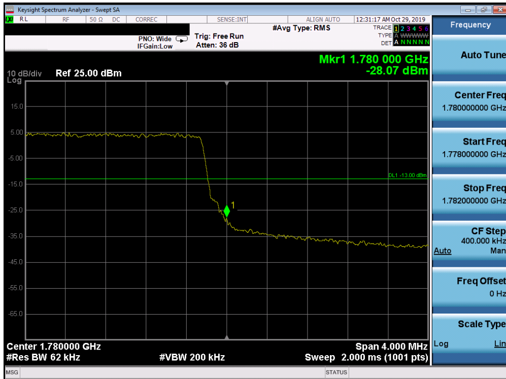
Plot 7-293. Upper Band Edge Plot (Band 66 - 5.0MHz QPSK - Full RB Configuration)
