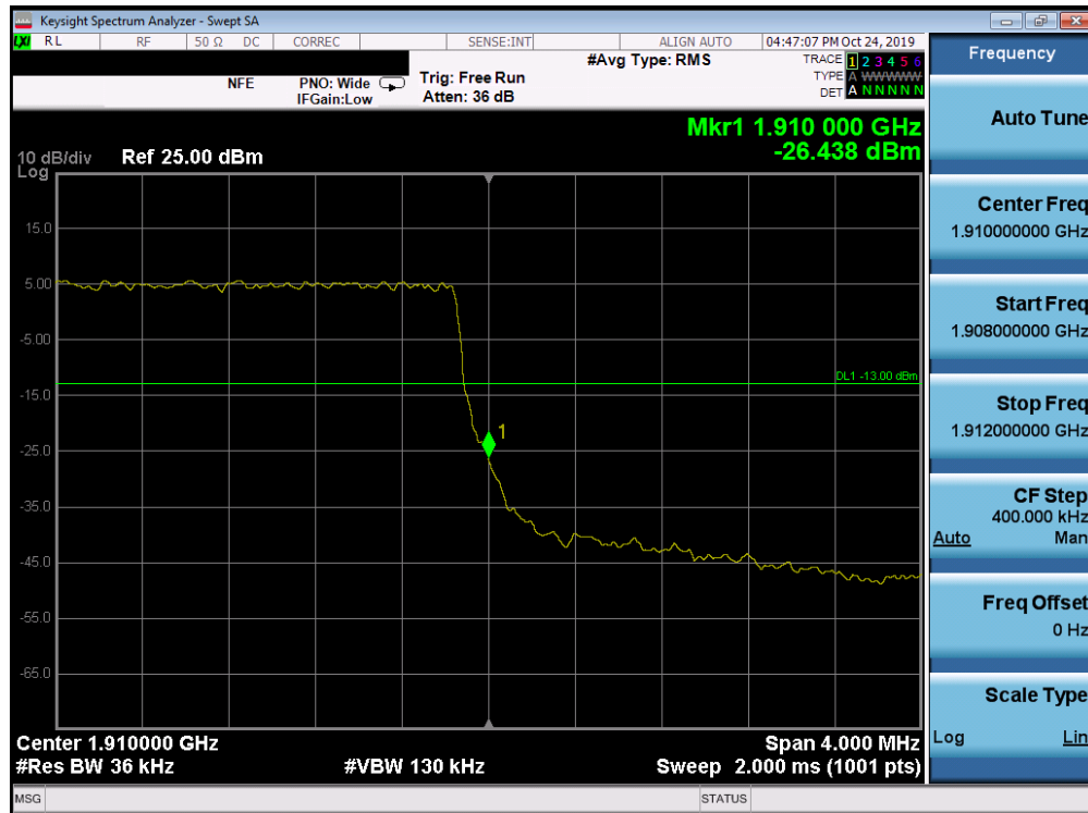
Plot 7-321. Upper Band Edge Plot (Band 2 - 3.0MHz QPSK - Full RB Configuration)
