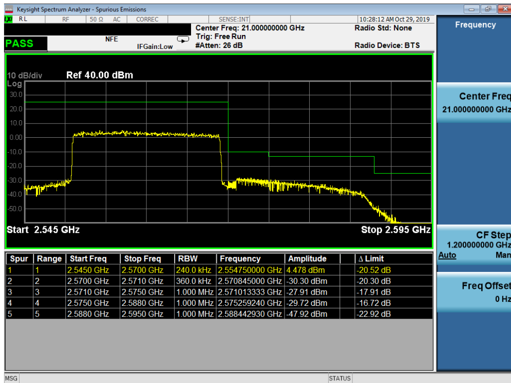
Plot 7-364. Upper ACP Plot (Band 7 - 20.0MHz QPSK - Full RB Configuration)
