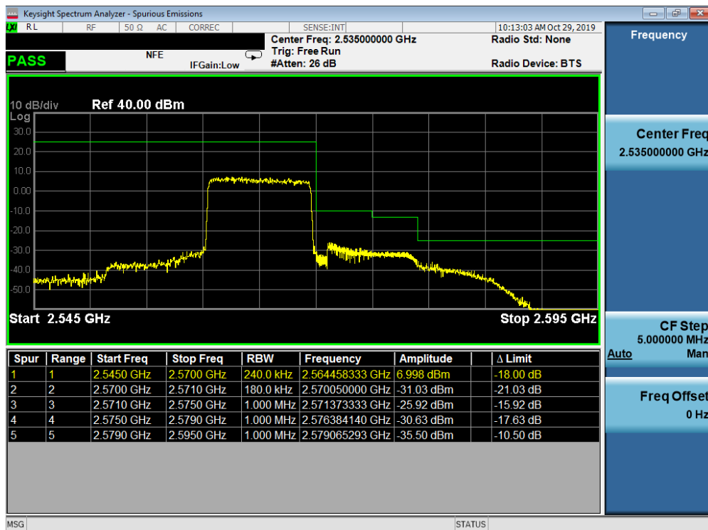
Plot 7-360. Higher ACP Plot (Band 7 - 10.0MHz QPSK - Full RB Configuration)
