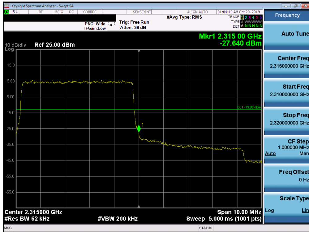
Plot 7-351. Upper Band Edge Plot (Band 30 - 5.0MHz QPSK - Full RB Configuration)
