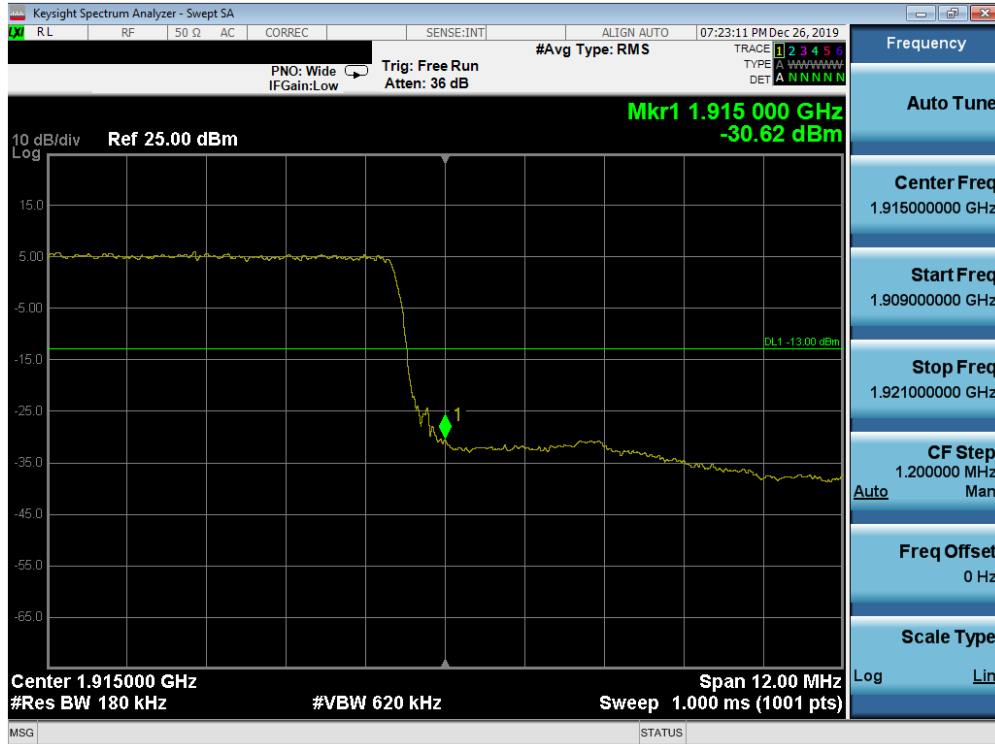
Plot 7-341. Upper Band Edge Plot (Band 25 - 15.0MHz QPSK - Full RB Configuration)
