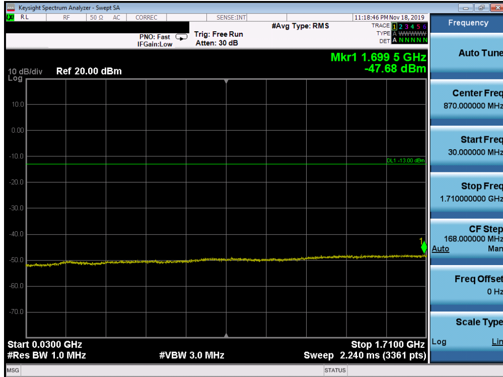
Plot 7-455. Conducted Spurious Plot (Band 66 – 20.0MHz QPSK – PCC 1/0 SCC 1/99 – High Channel)
