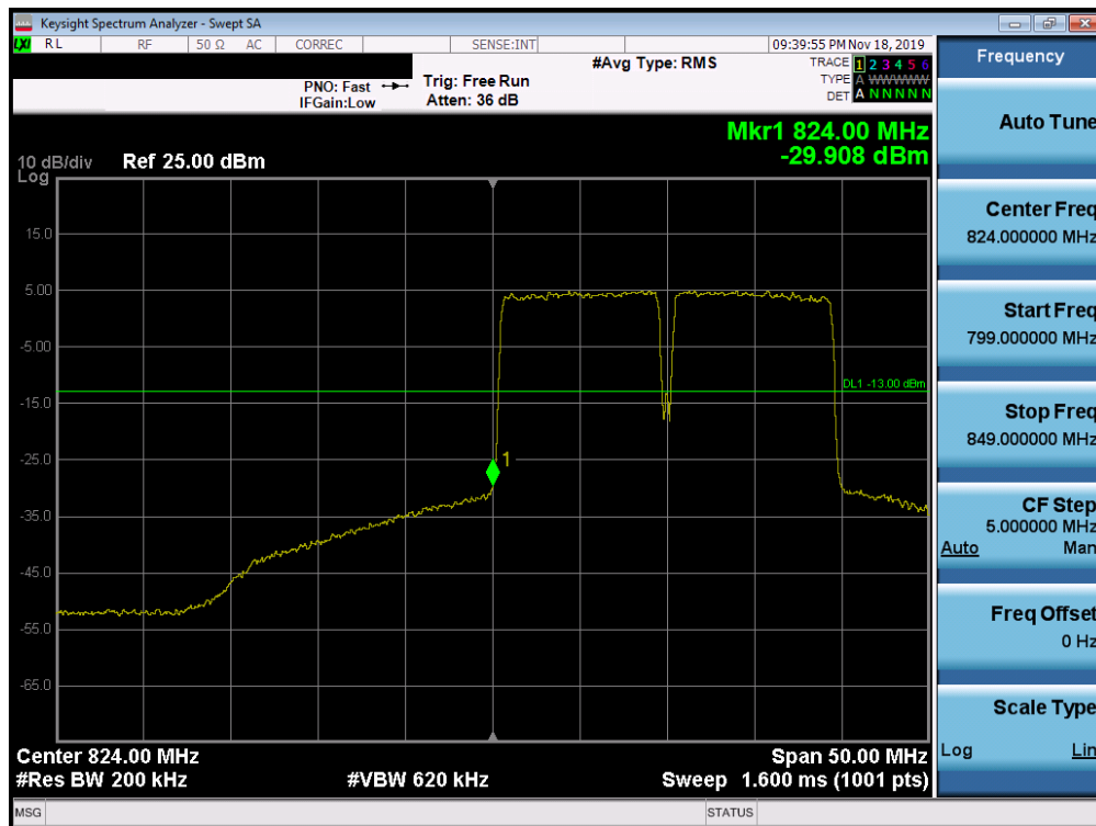
Plot 7-445. Lower Band Edge Plot (Band 5 QPSK – PCC:10 MHz SCC:10 MHz – Full RB)
