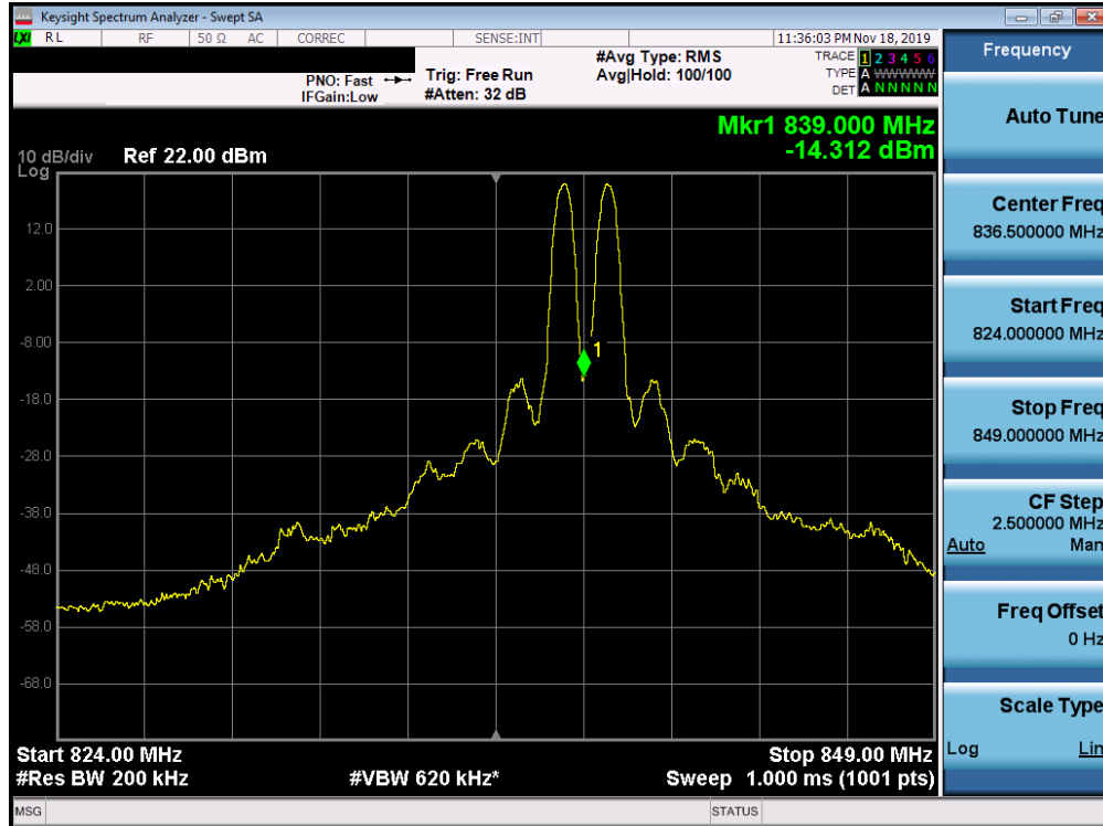
Plot 7-442. Conducted Spurious Plot (Band 5 – 10.0MHz QPSK – PCC 1/0 SCC 1/49 – High Channel)
