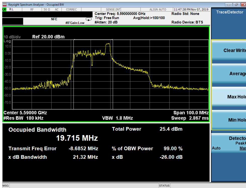
Plot 7-38. 26dB Bandwidth Plot SISO ANT2 (40MHz BW 802.11ax – 26 Tones (UNII Band 2C) – Ch. 118)
