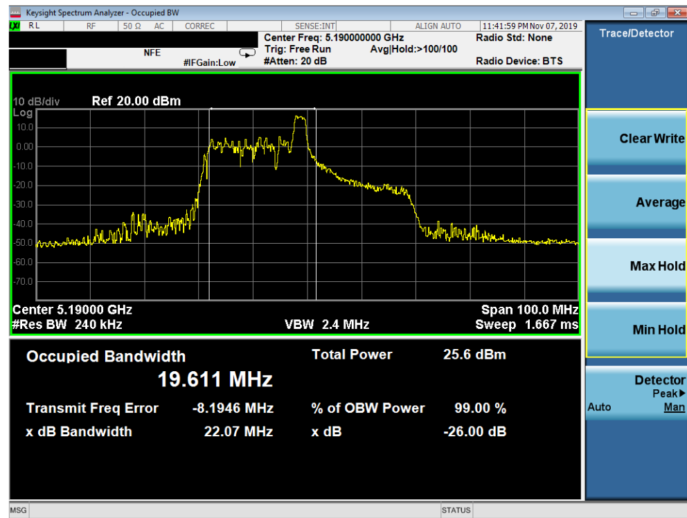
Plot 7-25. 26dB Bandwidth Plot SISO ANT2 (40MHz BW 802.11ax – 26 Tones (UNII Band 1) – Ch. 38)
