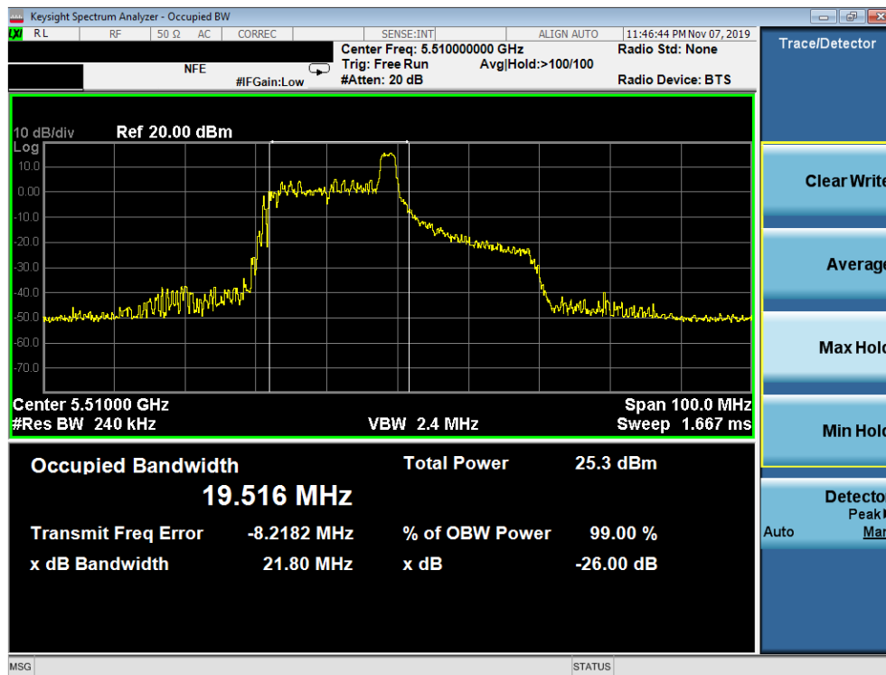
Plot 7-37. 26dB Bandwidth Plot SISO ANT2 (40MHz BW 802.11ax – 26 Tones (UNII Band 2C) – Ch. 102)
