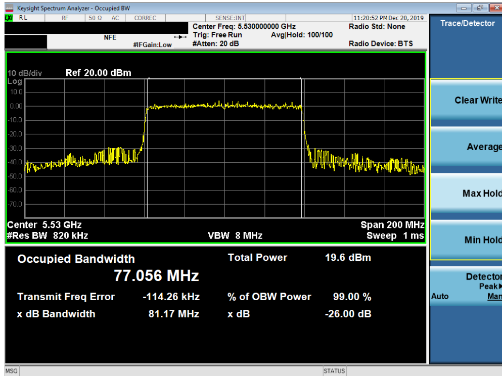
Plot 7-49. 26dB Bandwidth Plot SISO ANT1 (80MHz BW 802.11ax (UNII Band 2C) – Ch. 106)
