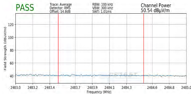
Plot 7-83. Radiated Restricted Upper Band Edge Measurement SISO ANT1 (Average – 242 Tones)
