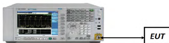
Figure 7-5. Test Instrument & Measurement Setup
