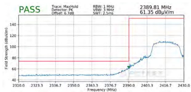
Plot 7-86. Radiated Restricted Lower Band Edge Measurement SISO ANT1 (Peak)
