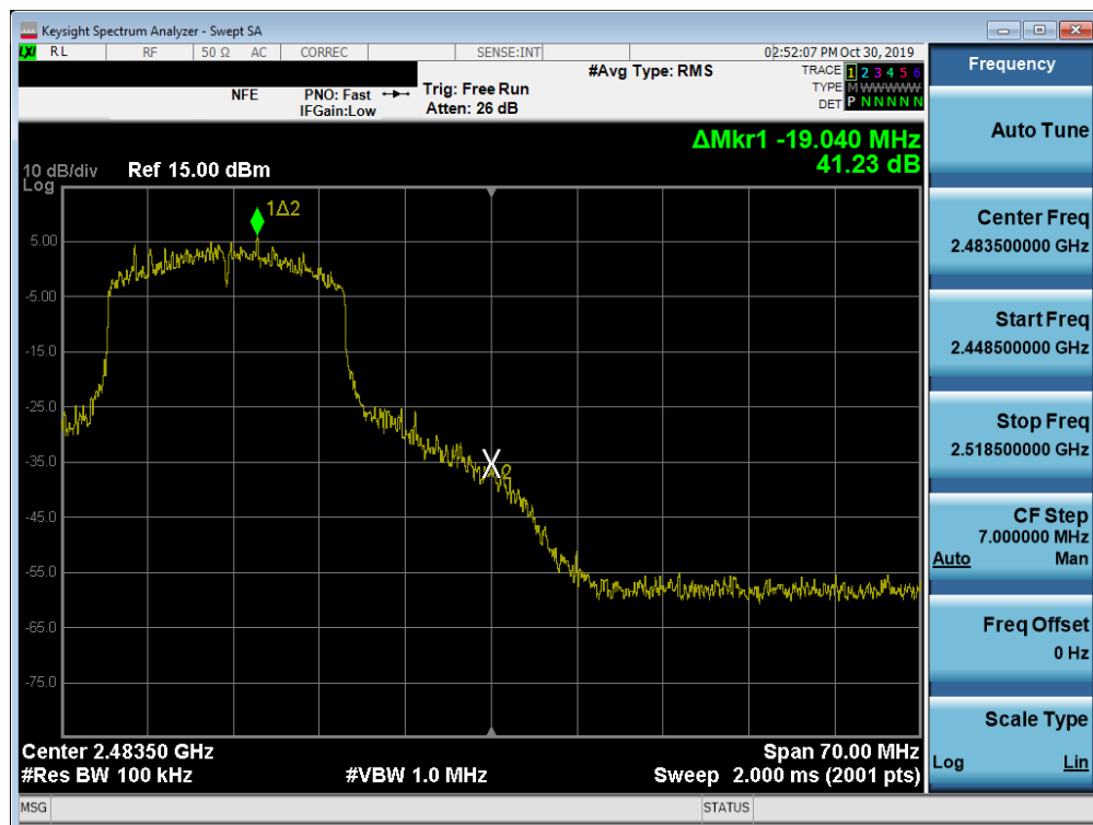
Plot 7-50. Band Edge Plot SISO ANT1 (802.11ax (2.4GHz) – Ch. 11)
