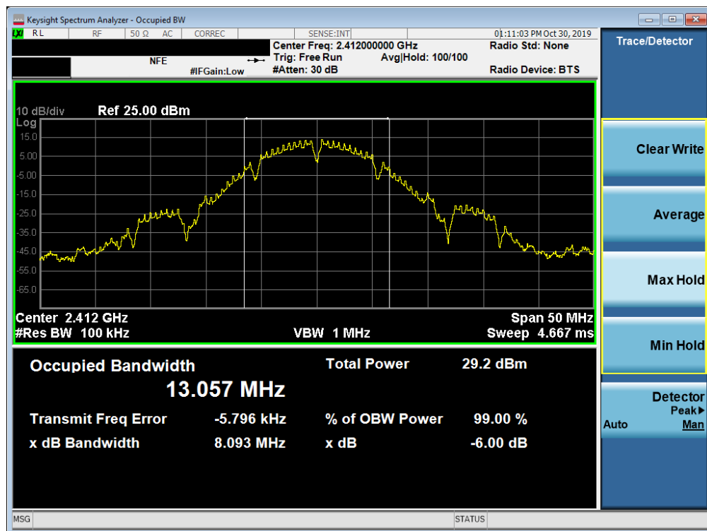
Plot 7-10. 6dB Bandwidth Plot SISO ANT1 (802.11b – Ch. 1)
