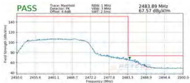
Plot 7-106. Radiated Restricted Upper Band Edge Measurement MIMO (Peak)
