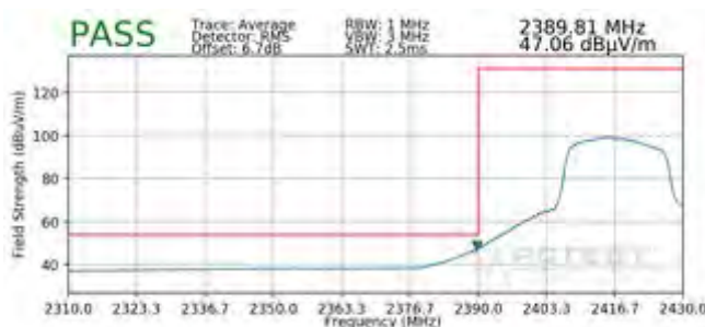
Plot 7-85. Radiated Restricted Lower Band Edge Measurement SISO ANT1 (Average)
