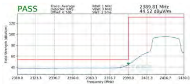
Plot 7-93. Radiated Restricted Lower Band Edge Measurement SISO ANT2 (Average)
