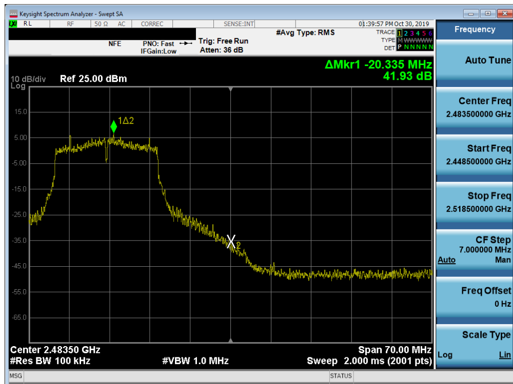
Plot 7-56. Band Edge Plot SISO ANT2 (802.11n (2.4GHz) – Ch. 11)
