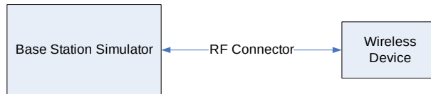
Figure 9-1 Power Measurement Setup
