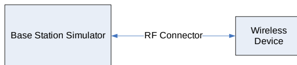
Figure 9-2 Power Measurement Setup
