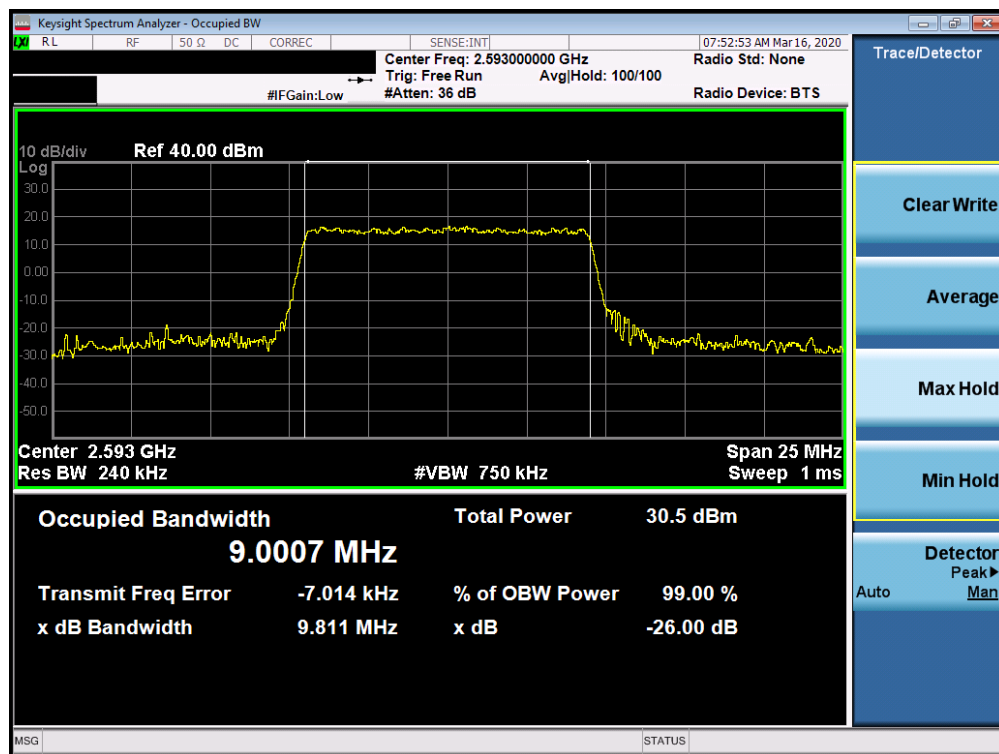
Plot 7-158. Occupied Bandwidth Plot (Band 41 - 10.0MHz 16-QAM - Full RB Configuration)
