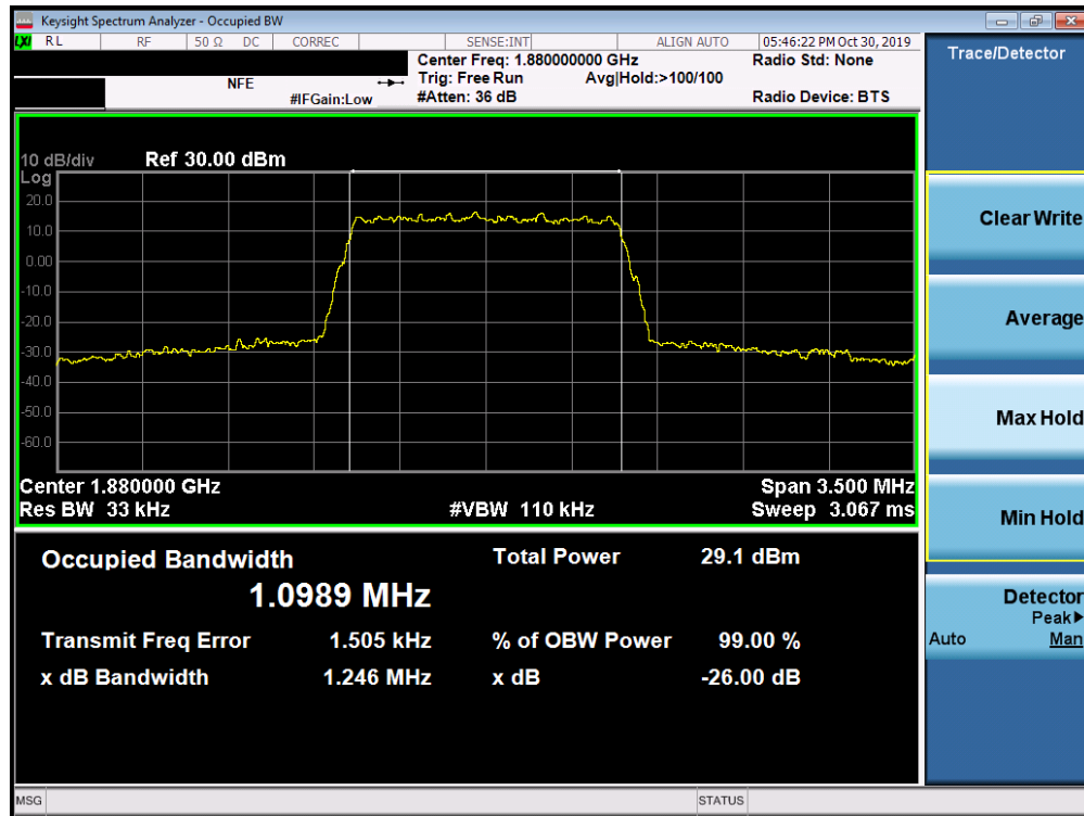
Plot 7-111. Occupied Bandwidth Plot (Band 2 – 1.4MHz 64-QAM - Full RB Configuration)
