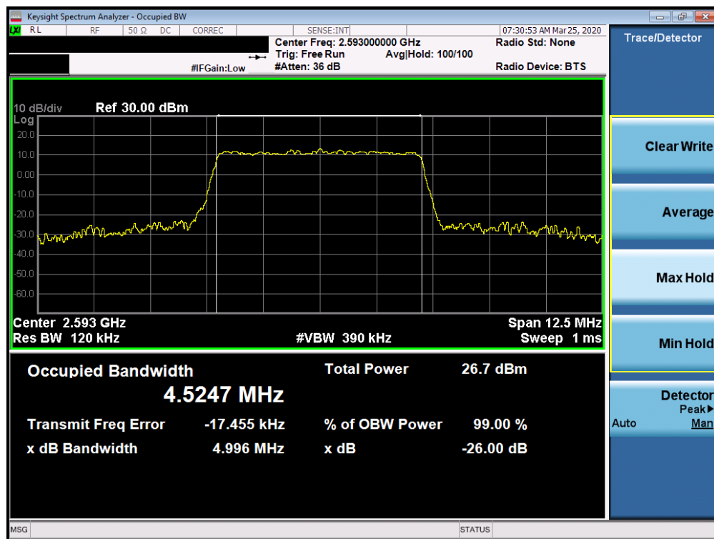
Plot 7-156. Occupied Bandwidth Plot (Band 41 - 5.0MHz 256-QAM - Full RB Configuration)
