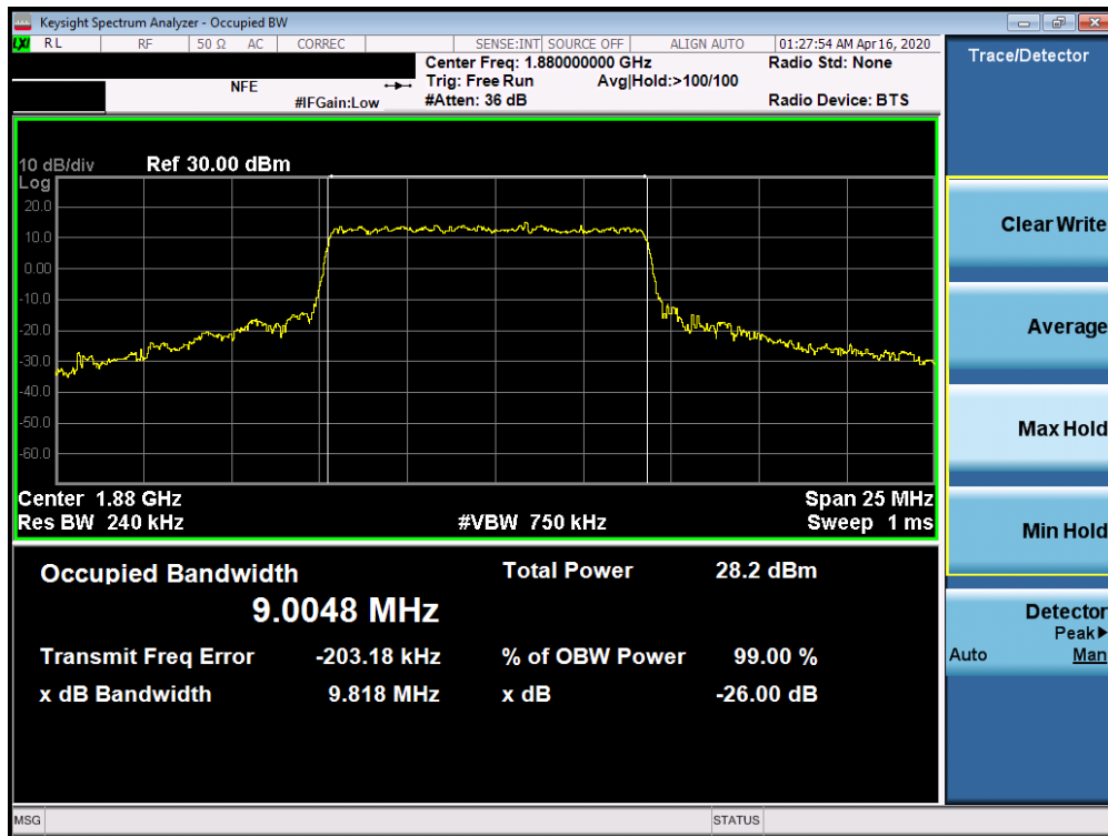
Plot 7-141. Occupied Bandwidth Plot (n2 - 10.0MHz CP-OFDM 64QAM - Full RB Configuration)
