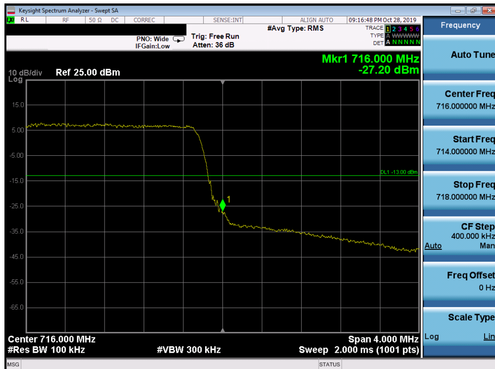
Plot 7-274. Upper Band Edge Plot (Band 12 - 5.0MHz QPSK - Full RB Configuration)
