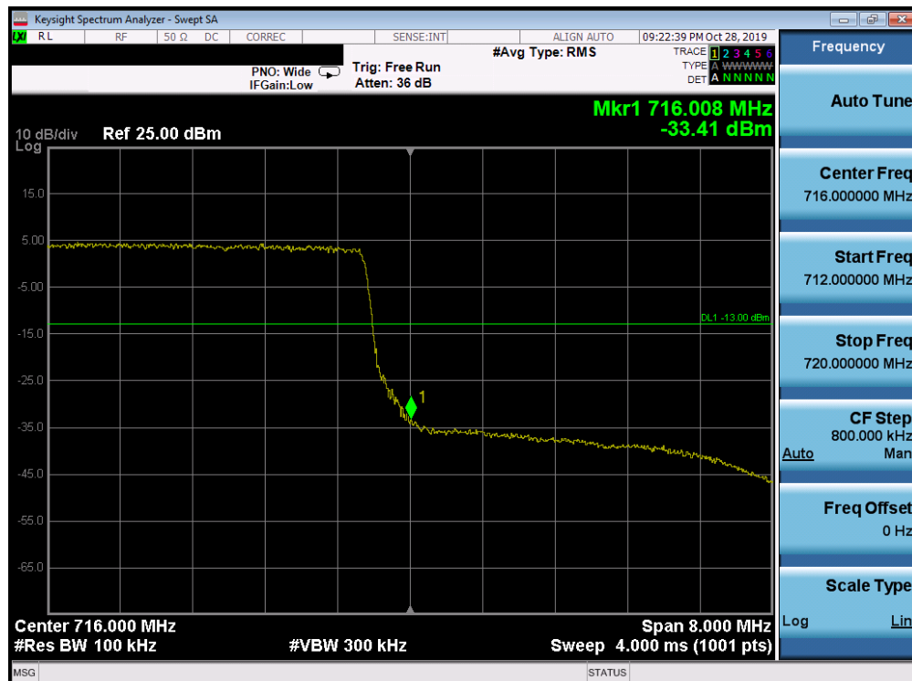
Plot 7-276. Upper Band Edge Plot (Band 12 - 10.0MHz QPSK - Full RB Configuration)
