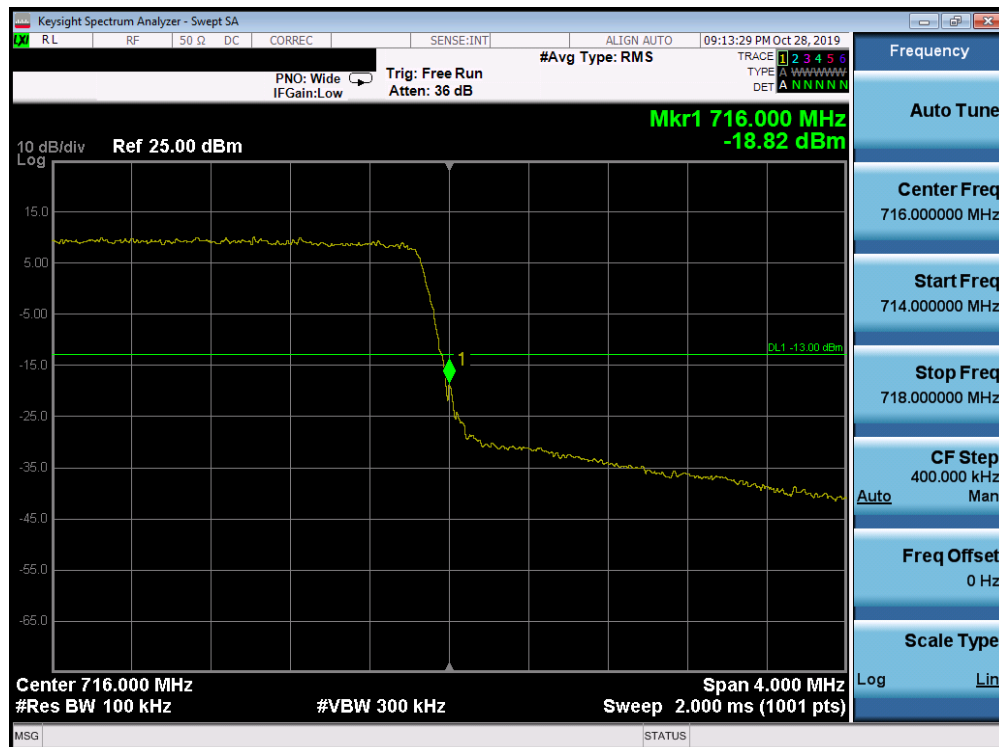
Plot 7-272. Upper Band Edge Plot (Band 12 - 3.0MHz QPSK - Full RB Configuration)
