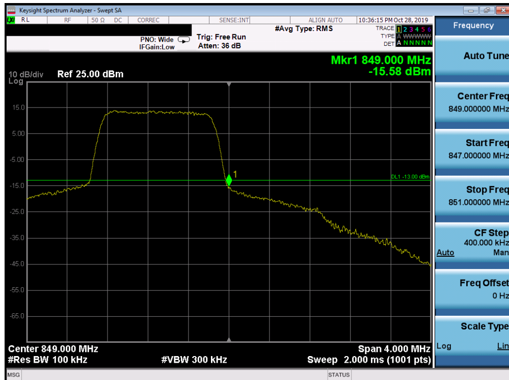
Plot 7-282. Upper Band Edge Plot (Band 26/5 - 1.4MHz QPSK - Full RB Configuration)
