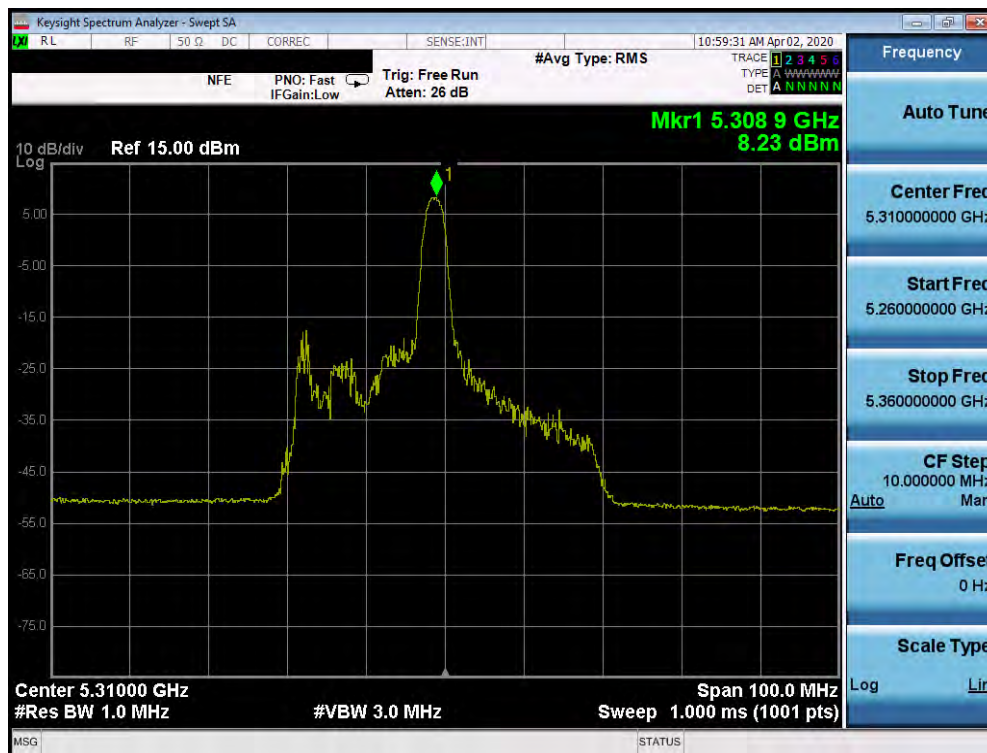
Plot 7-119. Power Spectral Density Plot SISO ANT1 (40MHz BW 802.11ax - 26 Tones (UNII Band 2A) - Ch. 62)
