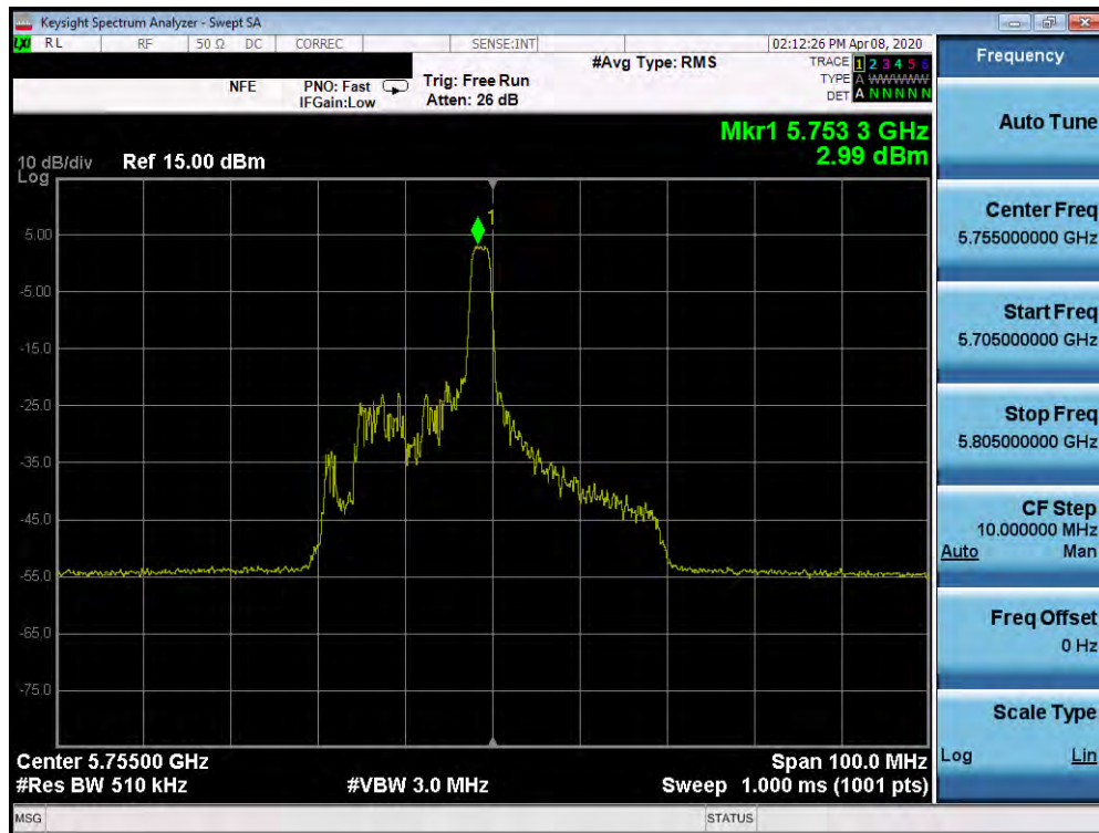
Plot 7-295. Power Spectral Density Plot MIMO ANT2 (40MHz BW 802.11ax - 26 Tones (UNII Band 3) - Ch. 151)
