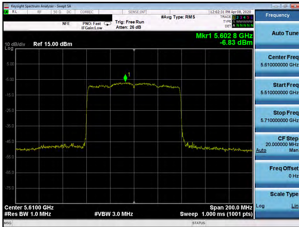
Plot 7-263. Power Spectral Density Plot MIMO ANT1 (80MHz BW 802.11ax – Full Tones (UNII Band 2C) – Ch. 122)
