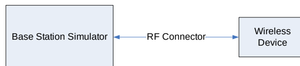
Figure 9-1 Power Measurement Setup
