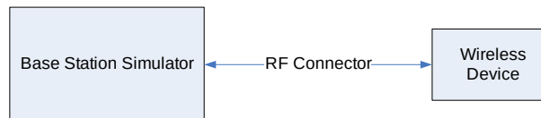
Figure 9-3 Power Measurement Setup
