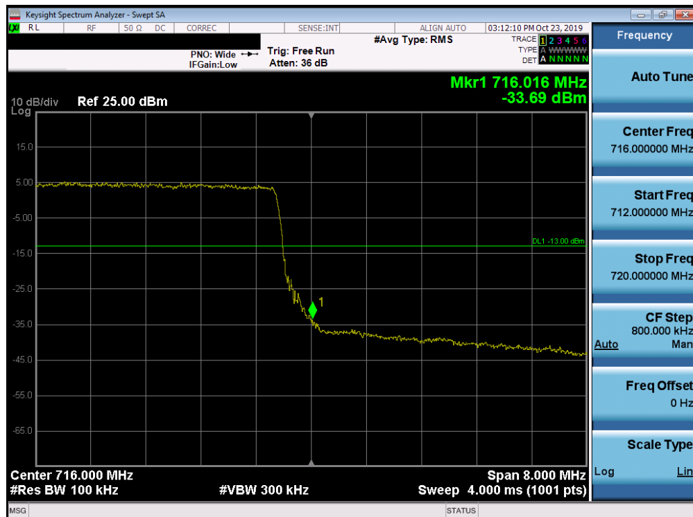
Plot 7-107. Upper Band Edge Plot (Band 12 - 10.0MHz QPSK - Full RB Configuration)
