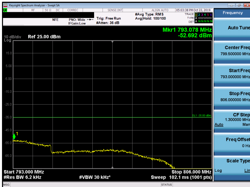
Plot 7-115. Upper Emission Mask Plot (Band 13 - 5.0MHz QPSK - Full RB Configuration)
