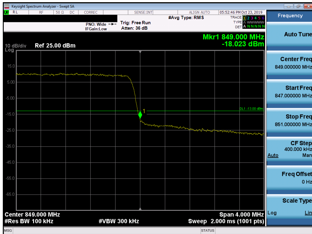
Plot 7-119. Upper Band Edge Plot (Band 5 - 3.0MHz QPSK - Full RB Configuration)
