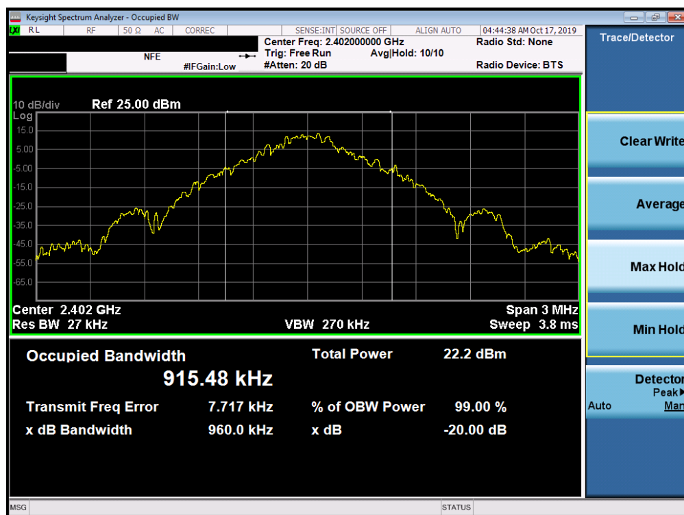
Plot 7-1. 20dB Bandwidth Plot (Bluetooth, 1Mbps – Ch. 0)
