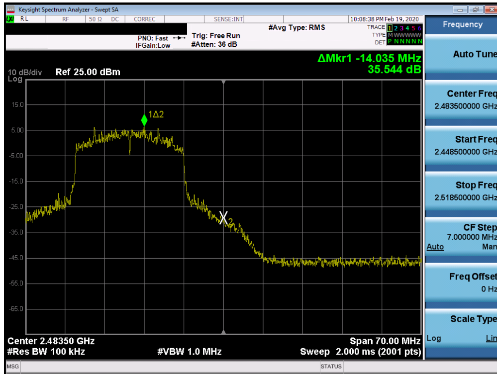
Plot 7-61. Band Edge Plot SISO ANT1 (802.11ax (2.4GHz) – Ch. 12)
